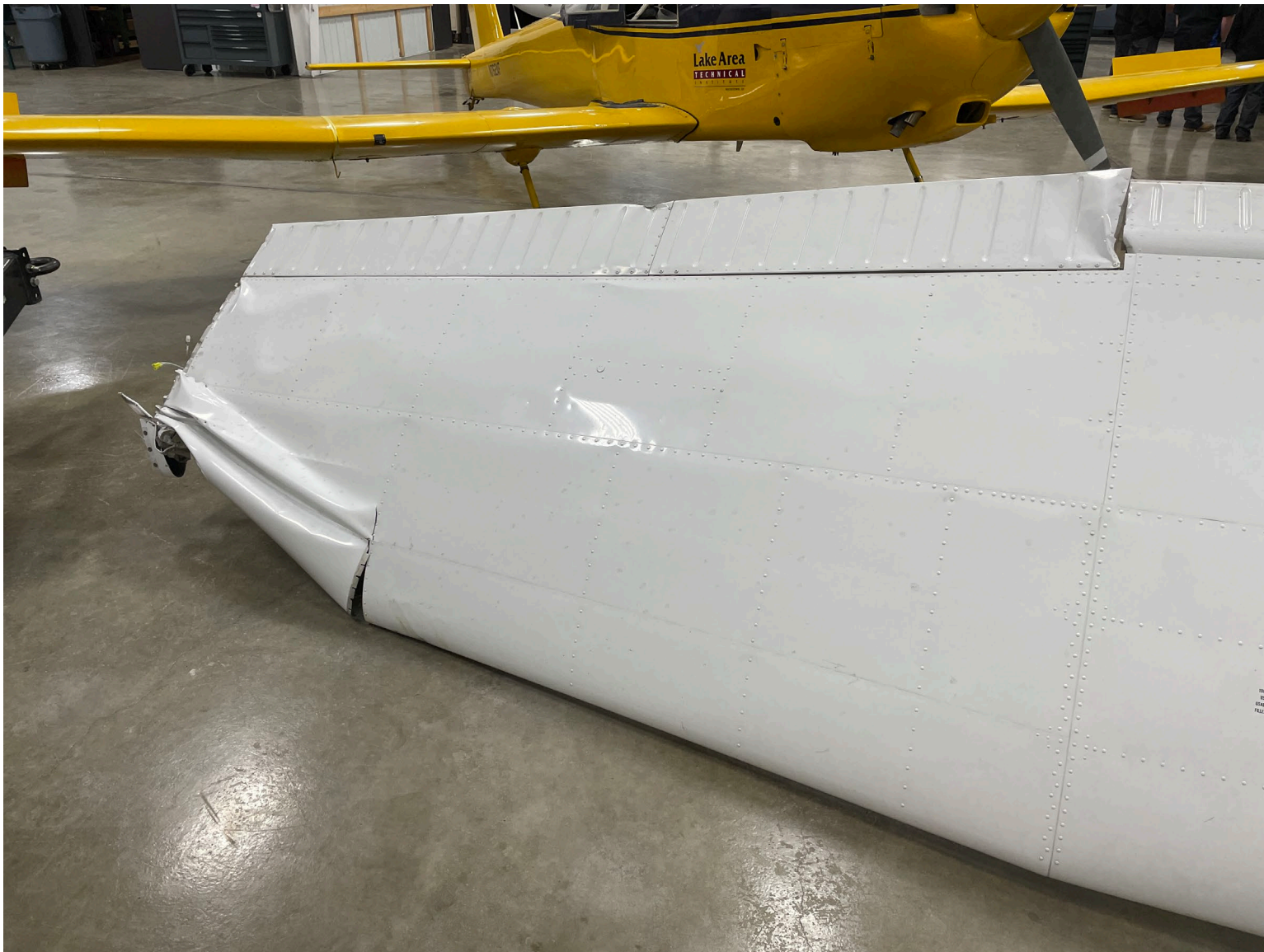
Photograph 2 - Right Wing Damage
