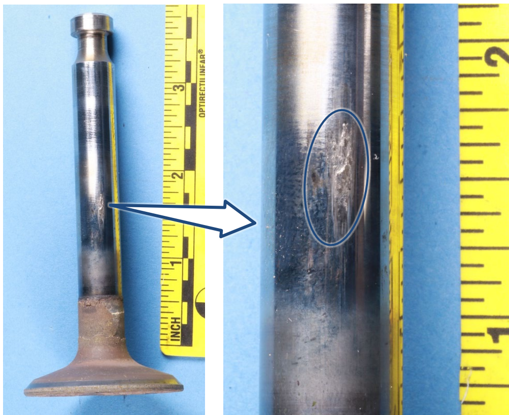
Figure 6. Exhaust valve showing raised deposits of smeared gray material (circled area) on the stem.
