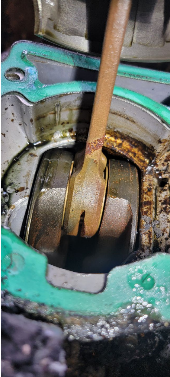
Figure 10. Rotec photo of connecting rod and crankshaft.
