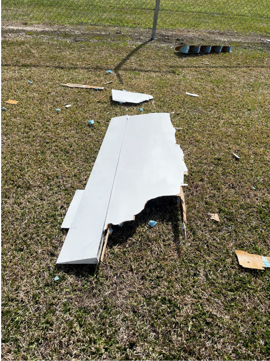
Figure 7. FAA Photo of the outboard aft portion of the left wing with aileron still attached.
