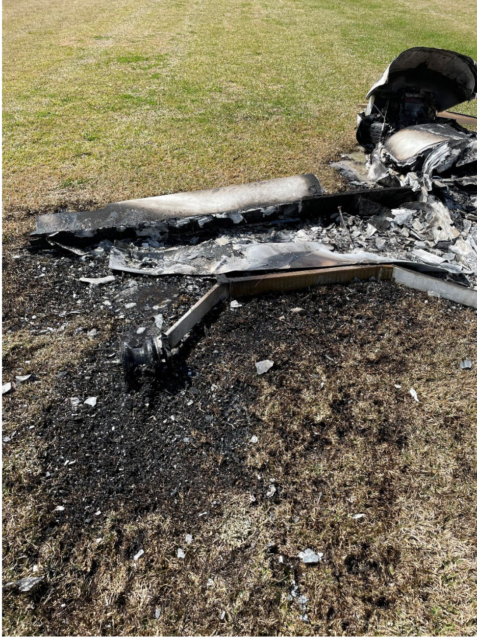
Figure 6. FAA Photo of the airplane's inboard left wing. Also visible is the separated main landing gear.
