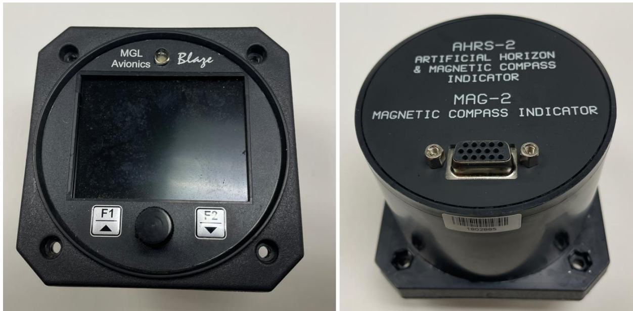
Figure 3. Front and back view of the MGL Blaze AHRS-2/MAG-2 as received.
