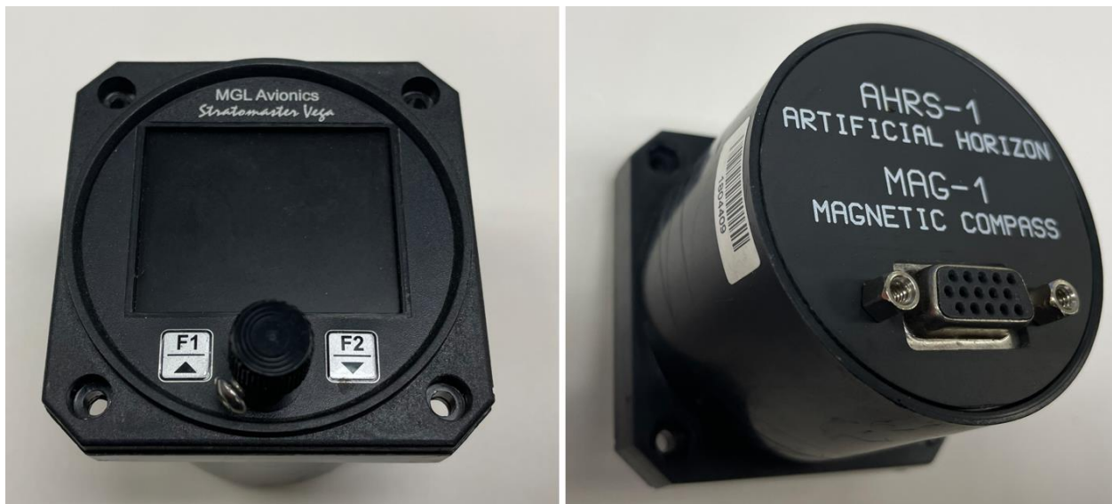
Figure 2. Front and back view of the MGL Stratomaster Vega AHRS-1/MAG-1 as received.
