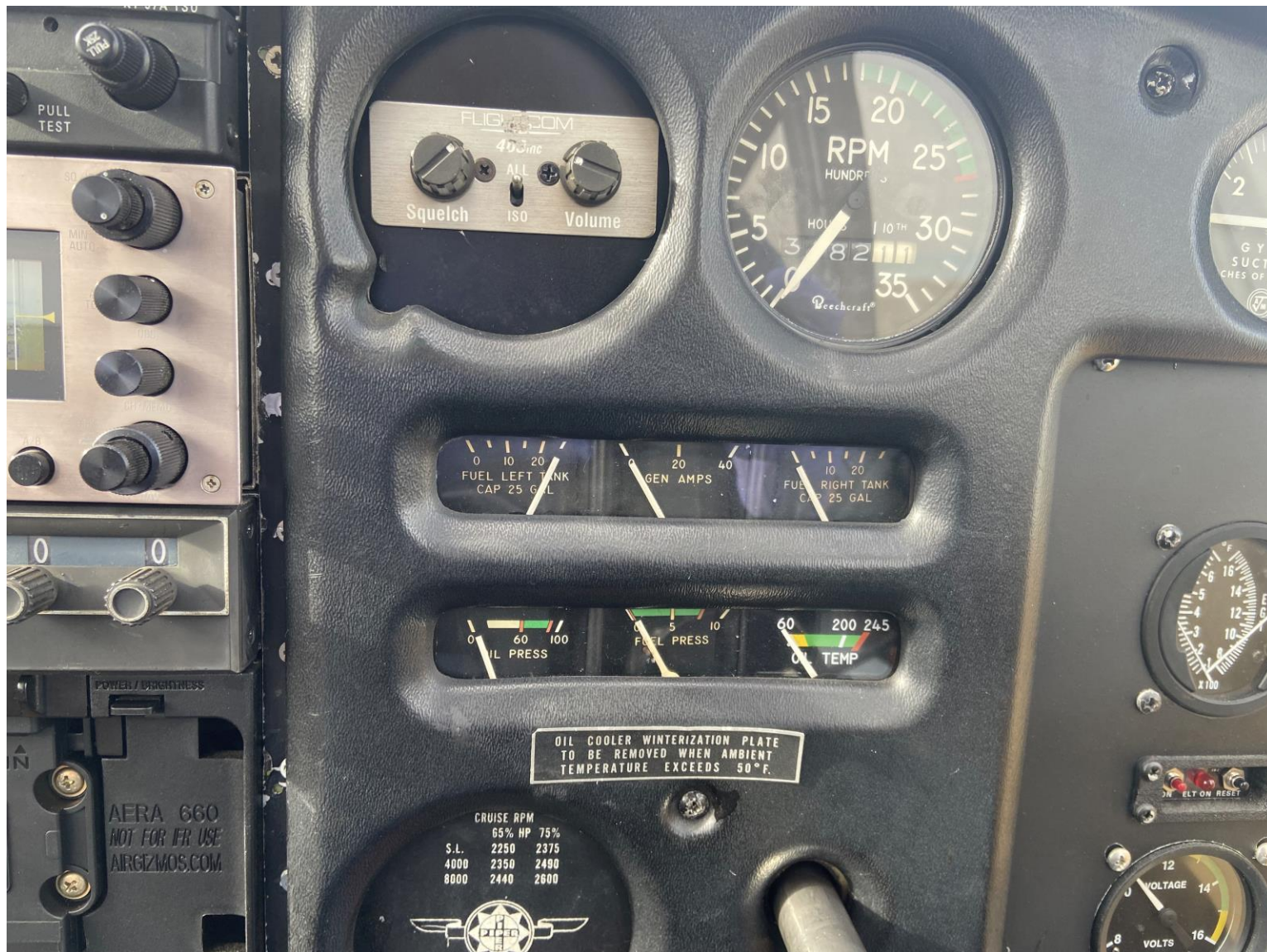
Photo 4 - Fuel gauges (Courtesy of FAA)
