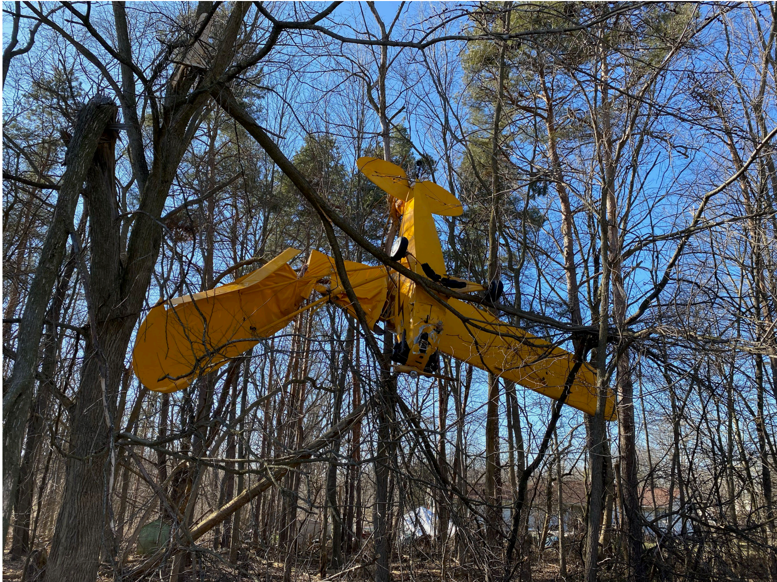
Photograph 3 - Damaged left wing and wing struts (Courtesy of FAA)
