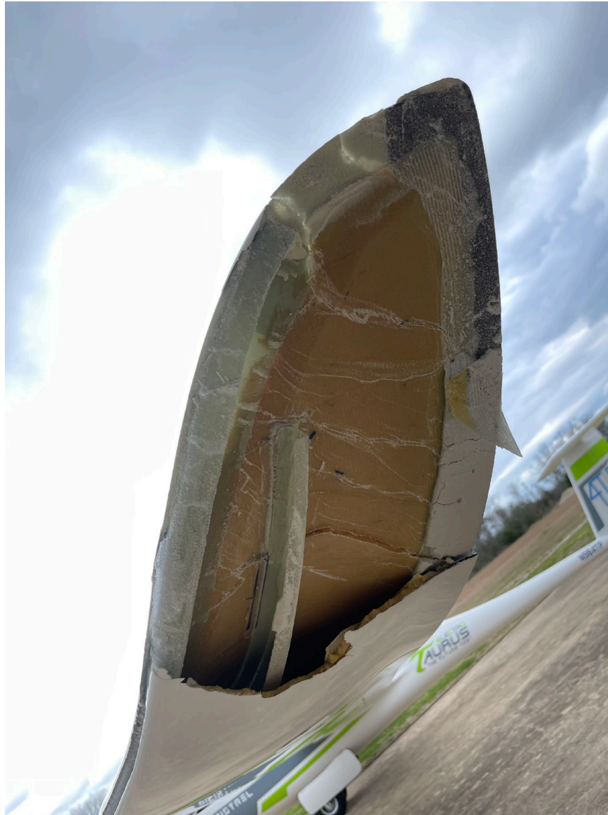
Photograph 2 - Pipistrel Glider with Damaged Left Wing (Courtesy of FAA)
