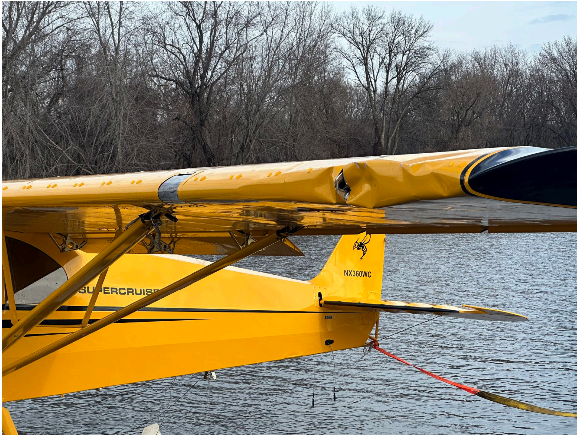
Photograph 2 - Wing damage - photo taken after recovery of airplane (Courtesy of a friend of pilot)
