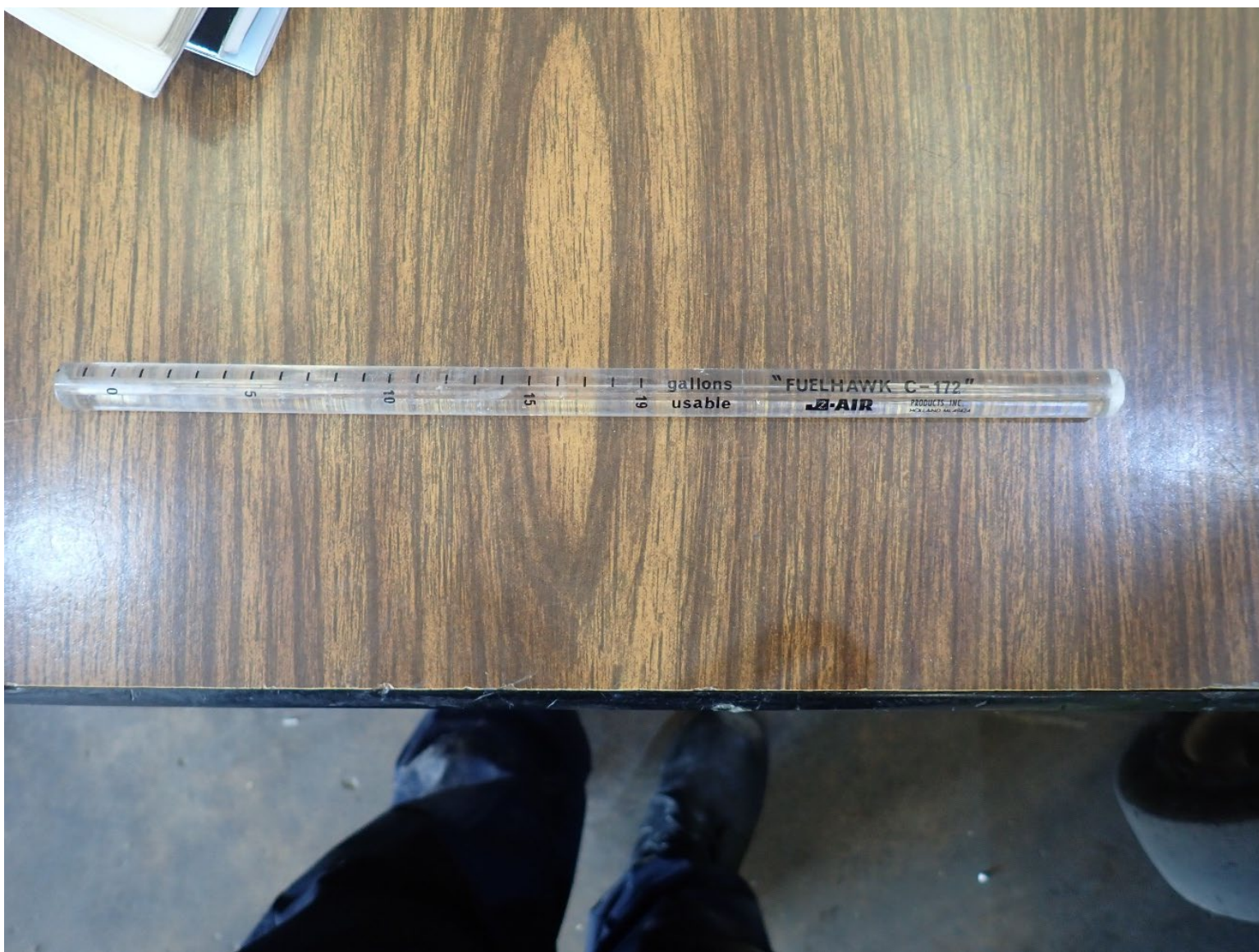
Photograph 9 - View of the fuel measuring stick found inside of the cockpit during the examination
