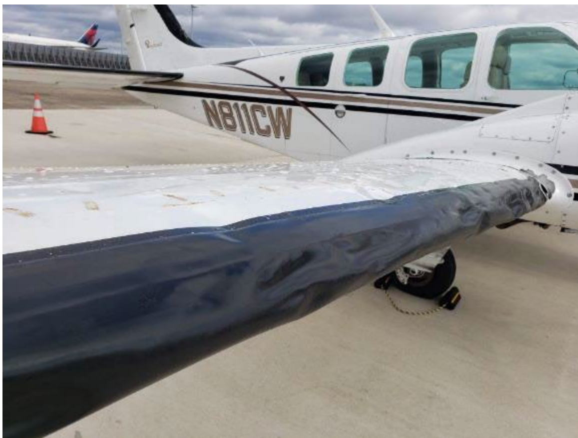
Photograph 1 - Accident airplane damage (Courtesy of FAA).
