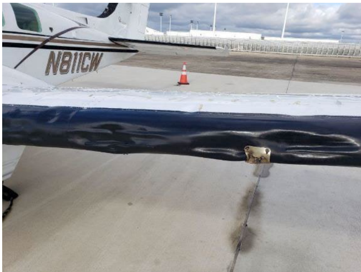
Photograph 3 - Left wing damage (Courtesy of FAA).
