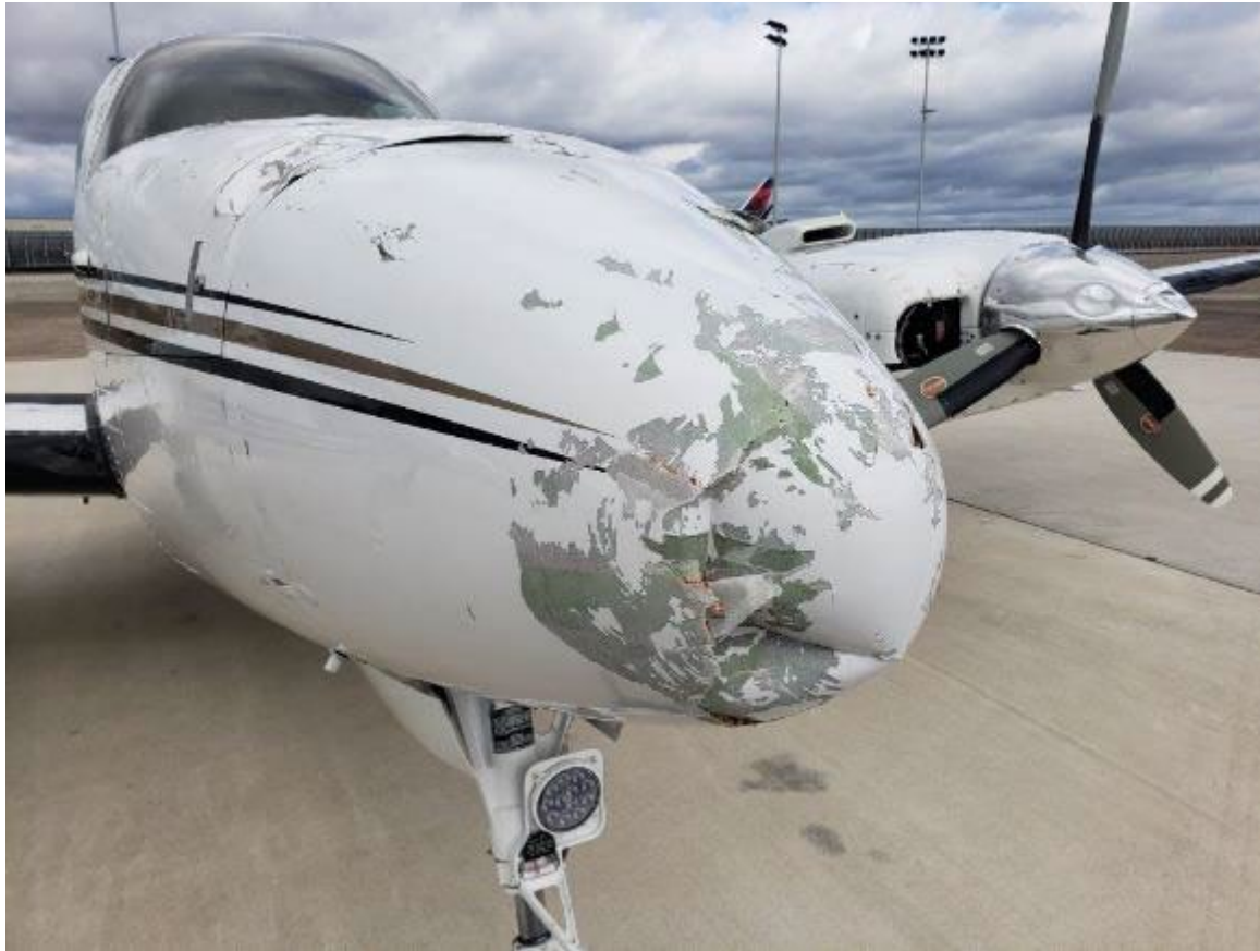
Photograph 2 - Damage to front of airplane (Courtesy of FAA).
