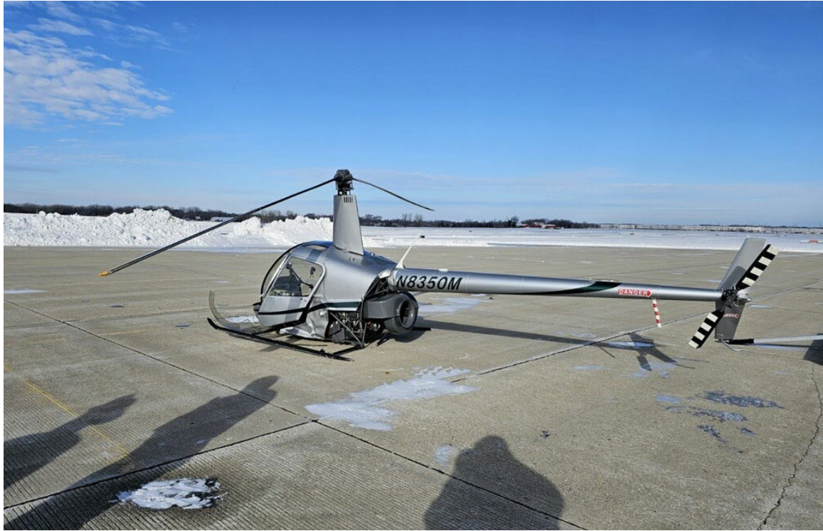
Photograph 1 - Deformation noted to the fuselage (Courtesy of Airport Manager)
