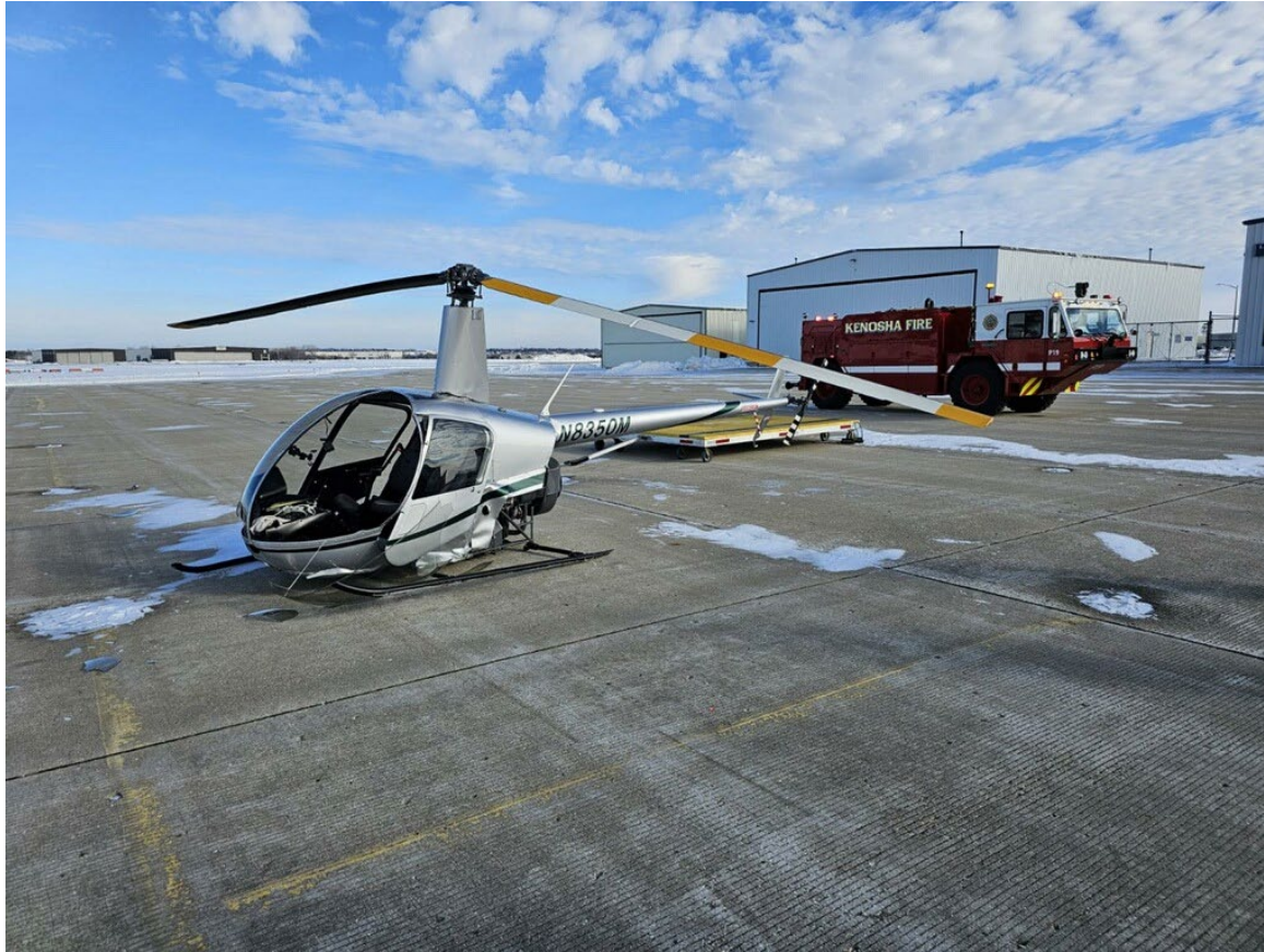
Photograph 2 - Deformation noted to main rotor blade (Courtesy of Airport Manager)
