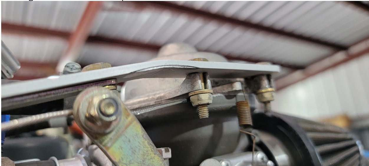
Figure 1: Right engine outboard throttle lever and rubbing.
