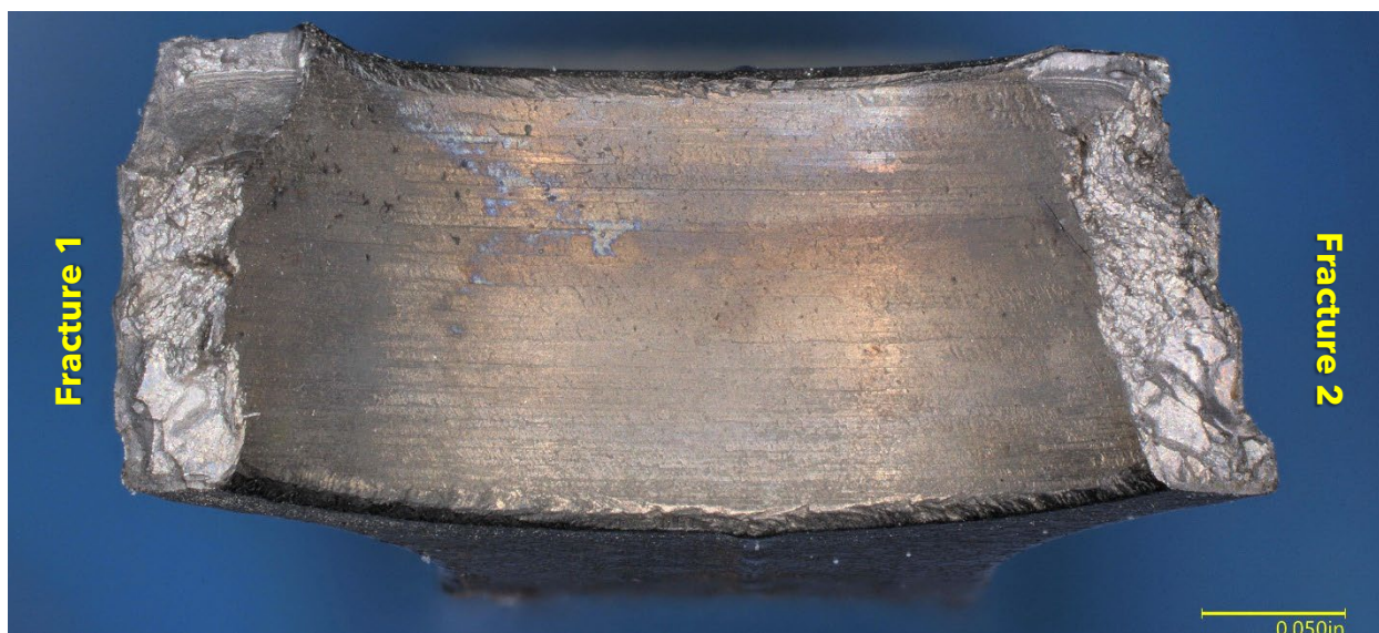
Figure 3. Mating fractures of the arms side, showing the bore of the actuating arm.
