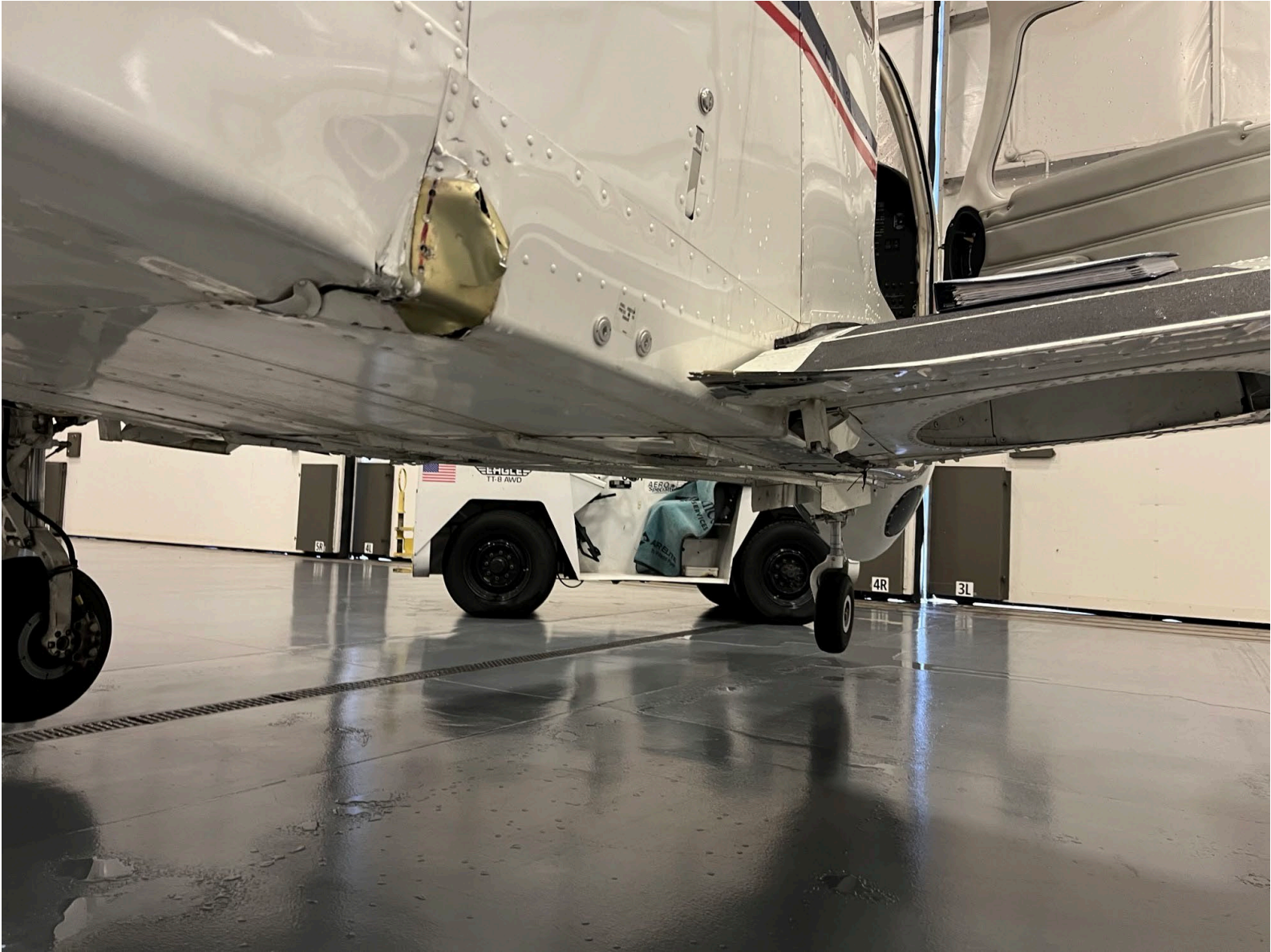
Photograph 3 - Lower fuselage and flap damage (Courtesy of FAA)
