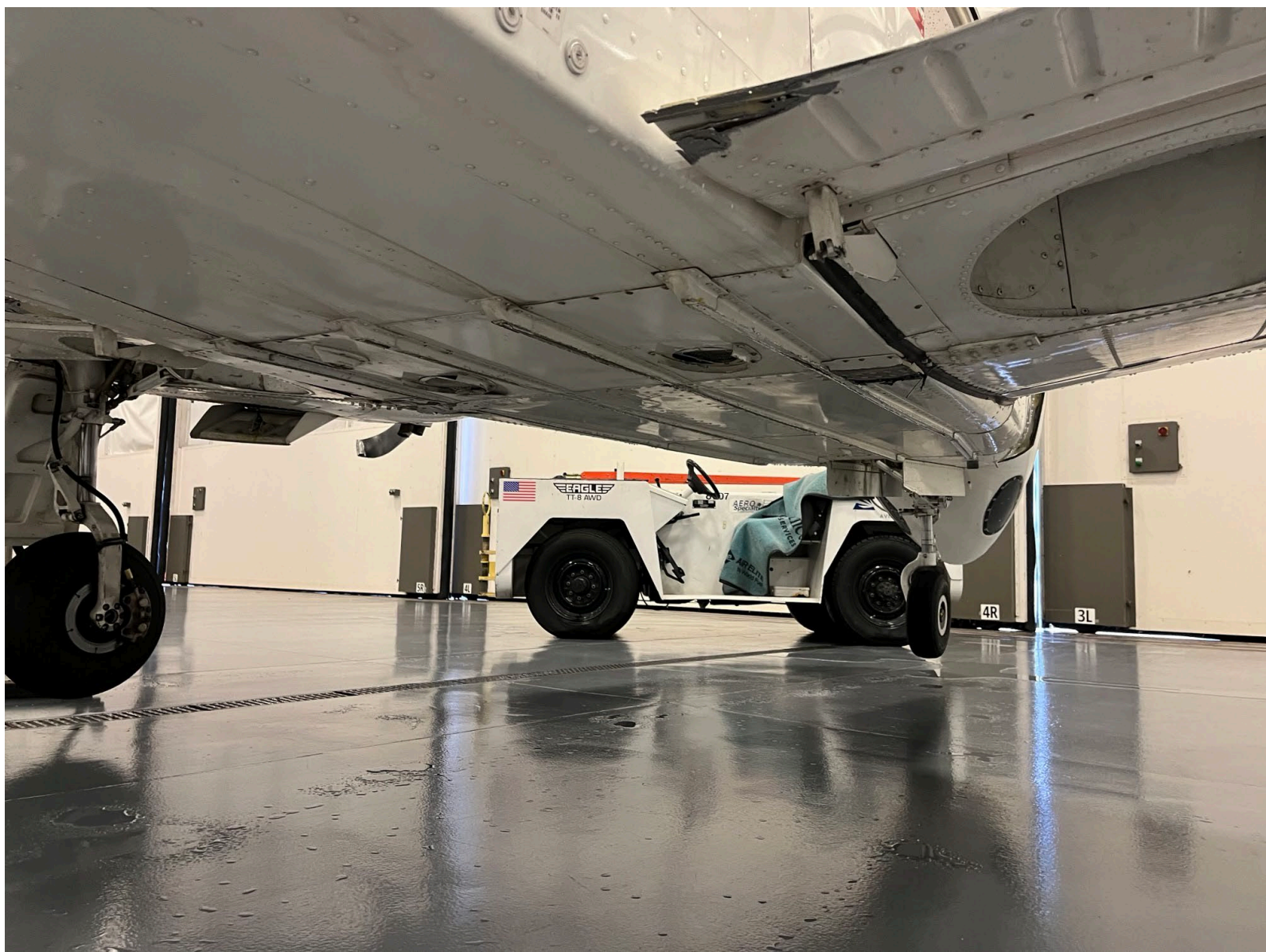
Photograph 4 - Lower fuselage and flap damage (Courtesy of FAA)
