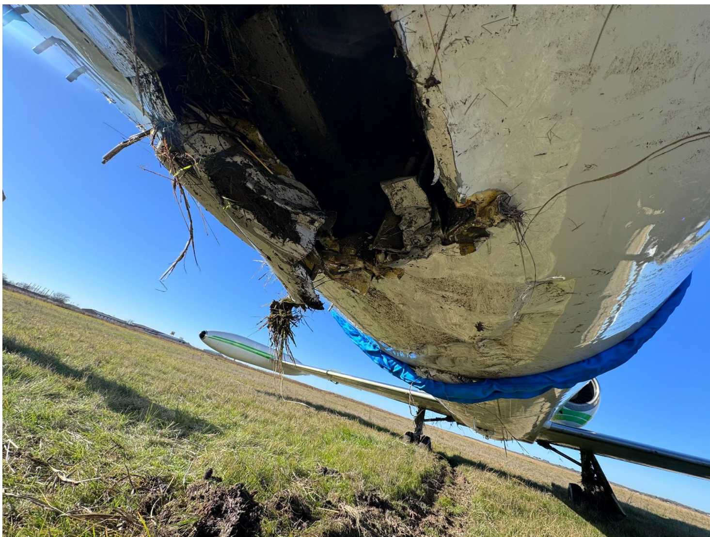
Photograph 2 - Belly Damage (Courtesy of FAA)
