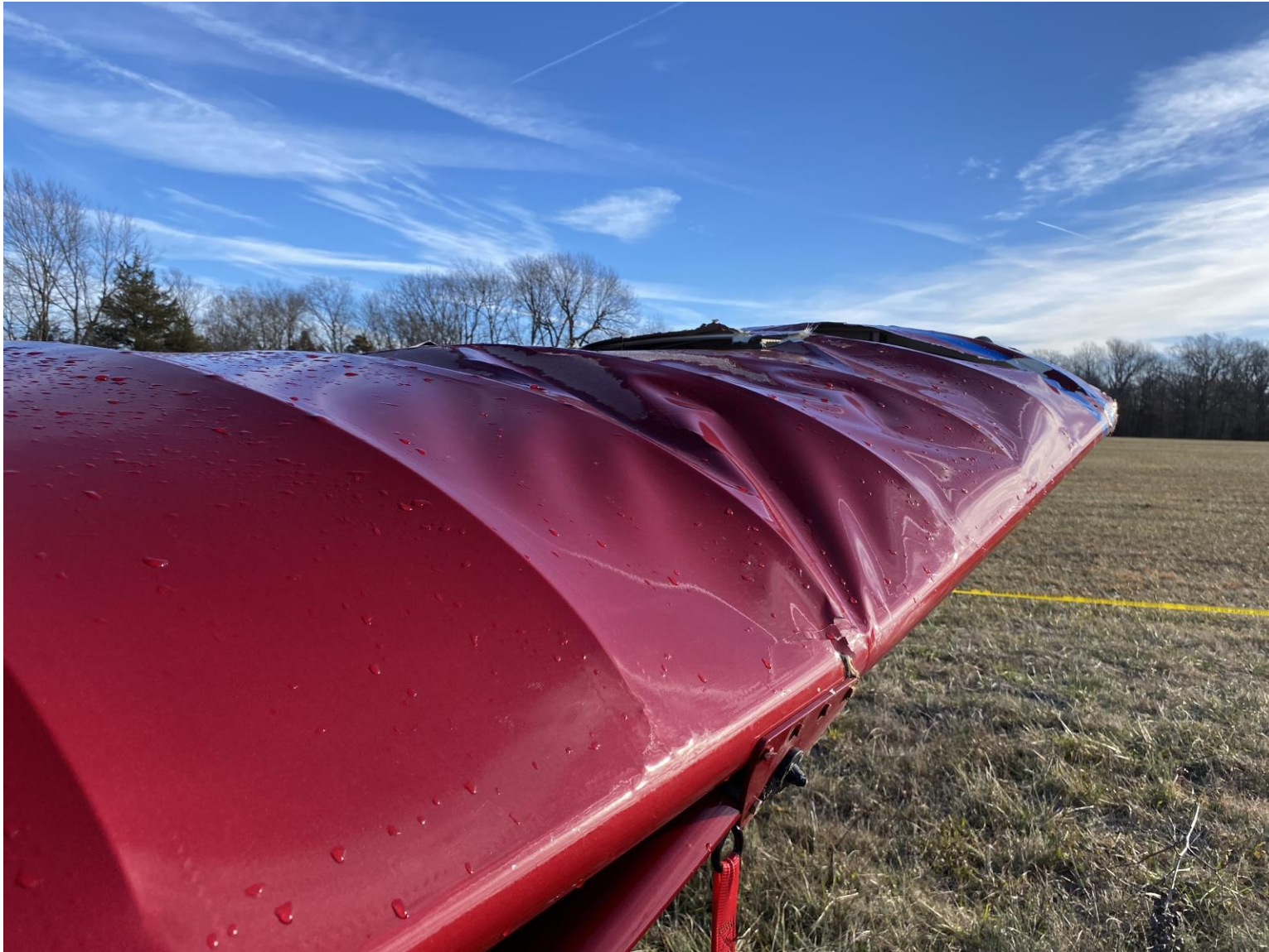
Photo 4 - Right wing damage (Courtesy of FAA)
