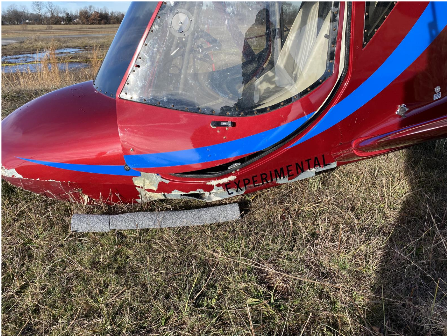
Photo 3 - Forward fuselage damage (Courtesy of FAA)
