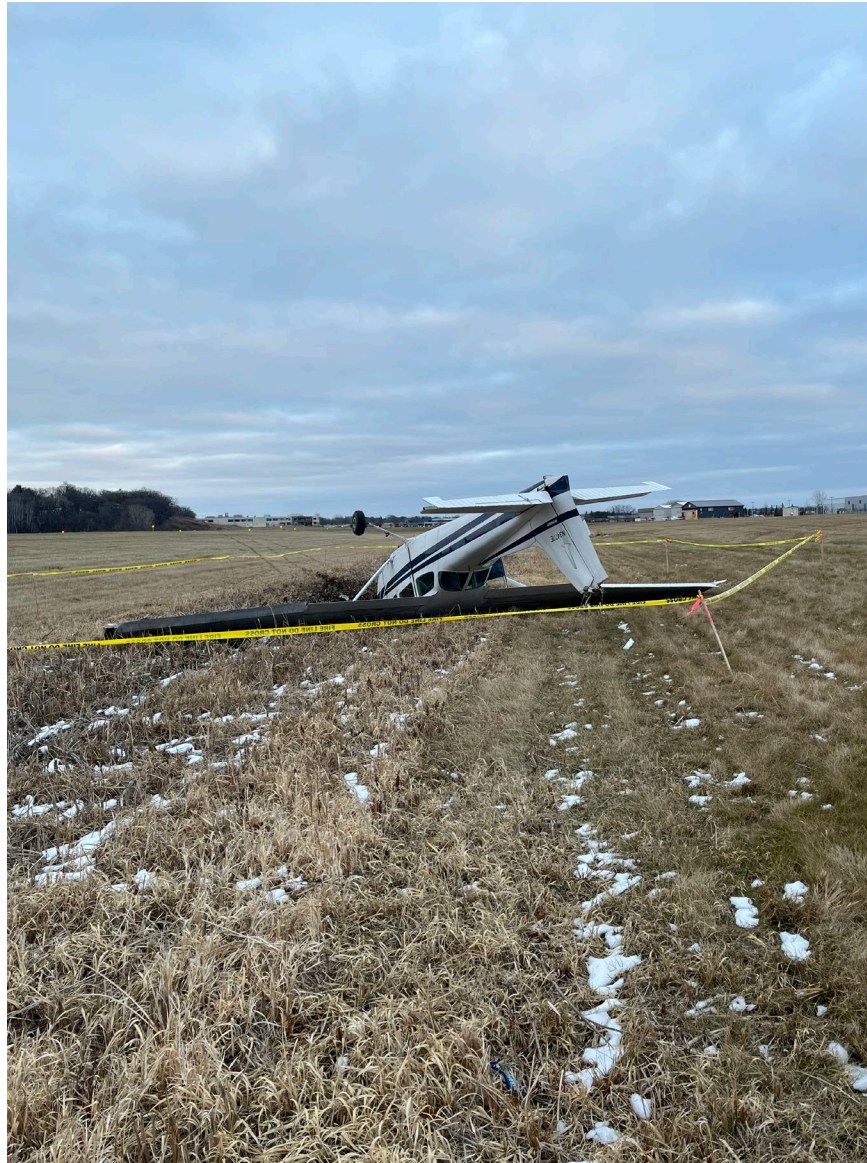
Photograph 1 - Deformation noted to rudder (Courtesy of FAA)
