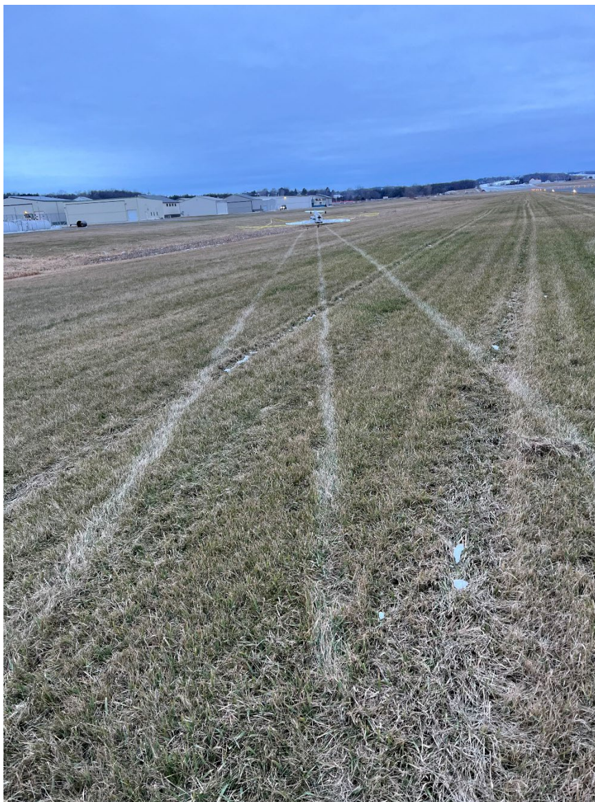
Photograph 2 - Wheel impression noted from the runway to the wreckage (Courtesy of FAA)
