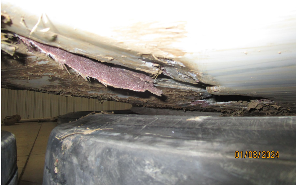
Photograph 2 - Damage to wing (Courtesy of FAA)
