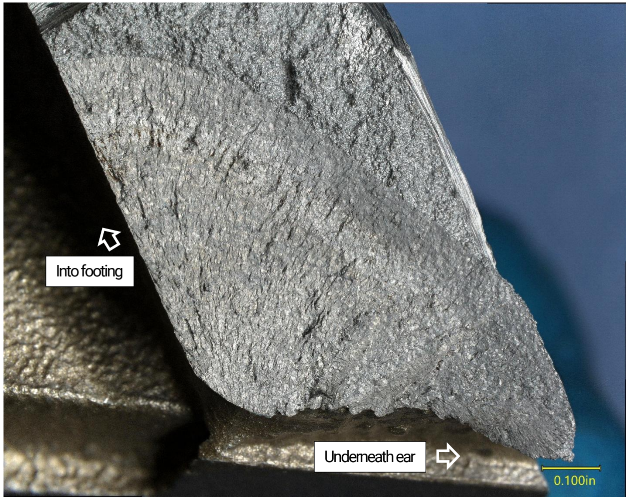
Figure 11. One of the crack surfaces after cleaning. The features were consistent with high-cycle fatigue.
