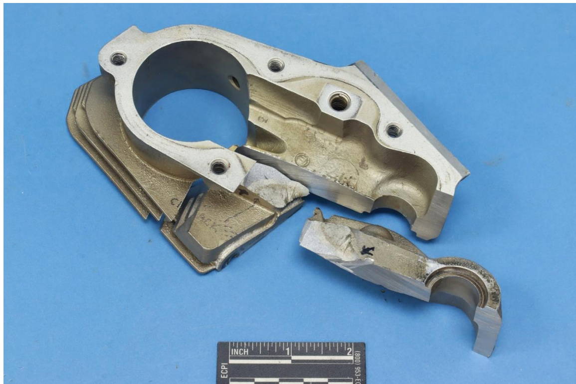
Figure 10. a) Exhaust valve rocker box region sectioned from the rest of the cylinder and b) further sectioning and exposure of the crack.
