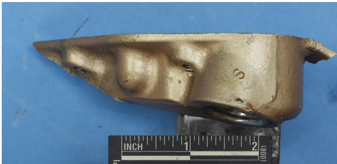
Figure 5. a) Overview image of cylinder, serial number AC16KA158, with fractured exhaust rocker box ear and b) image of fractured ear showing stamp mark.
