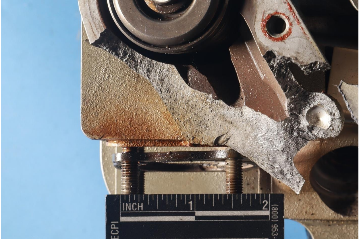
Figure 2. Fatigue fracture starting at the outer edge of the lower corner of the exhaust rocker box footing.
