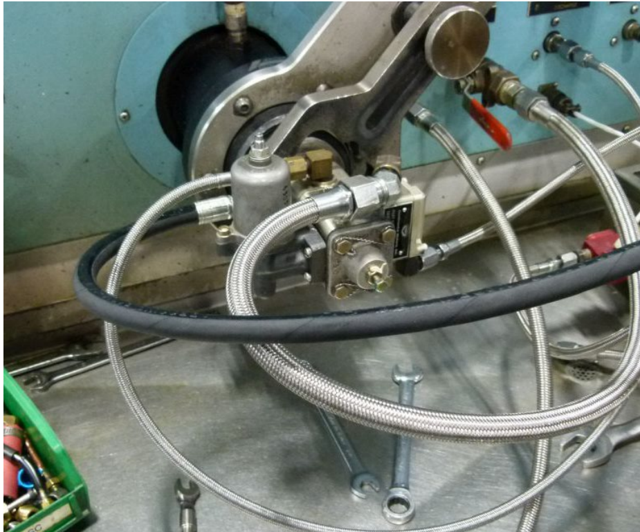
Figure 2 - Fuel Pump (installed on test bench)
