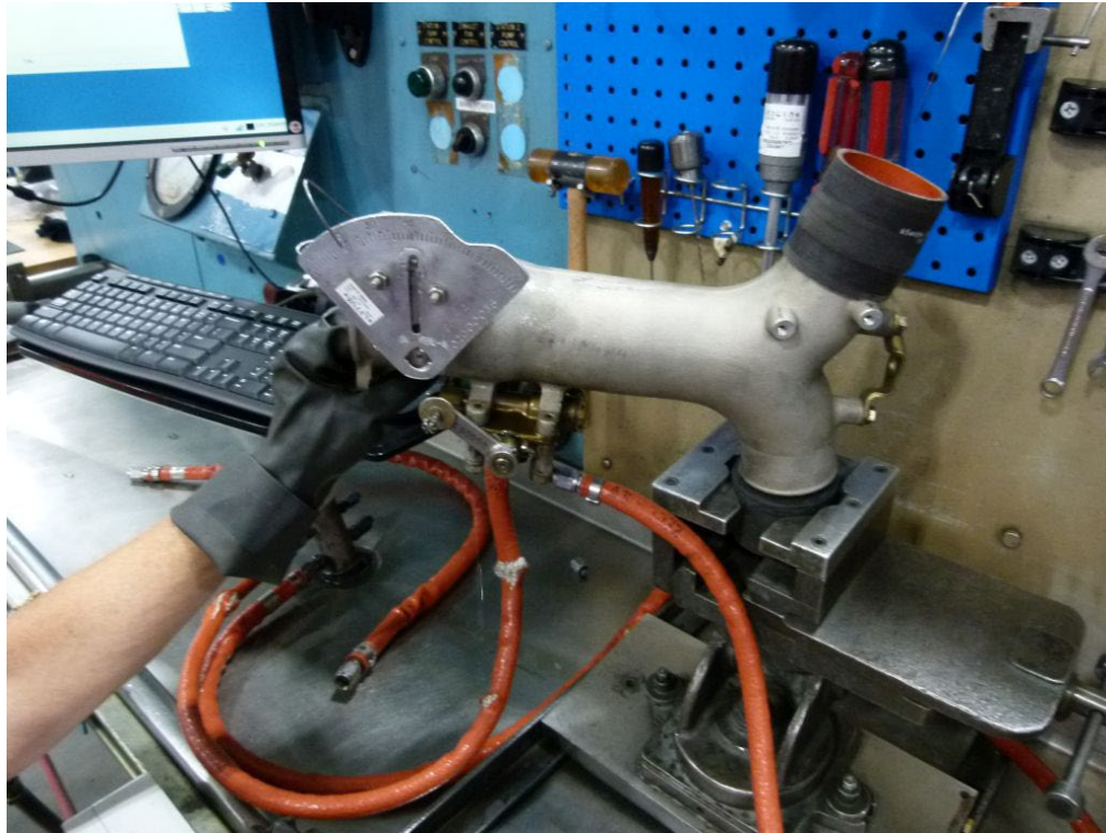
Figure 6 - Throttle Unit (installed on test bench)
