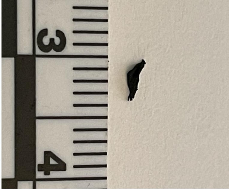
Figure 4 - Fuel Pump Debris
