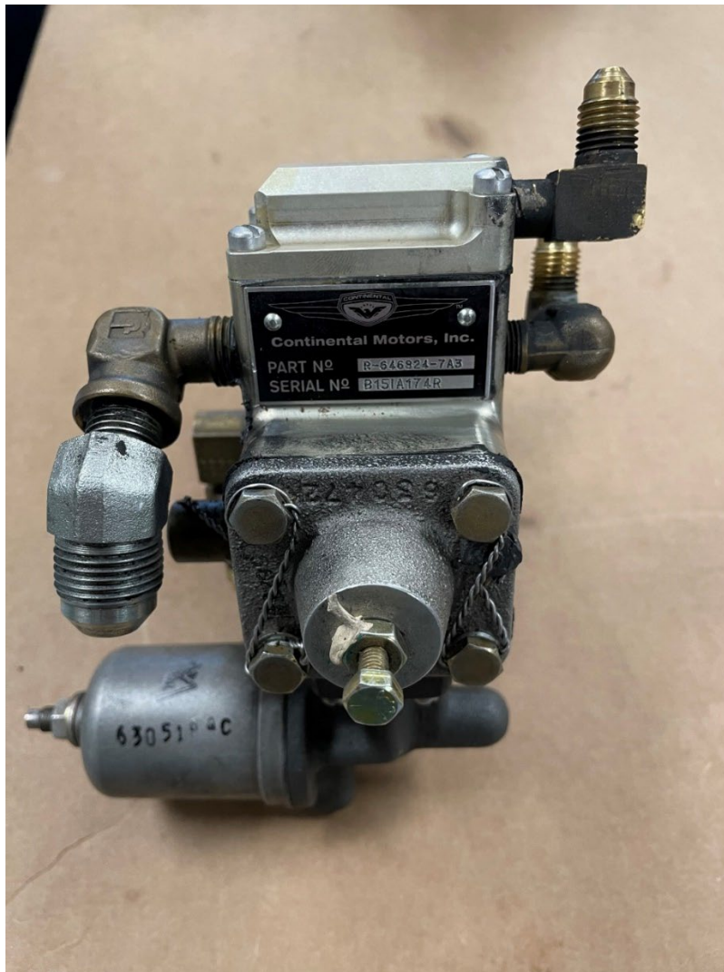
Figure 1 - Fuel Pump (as received)
