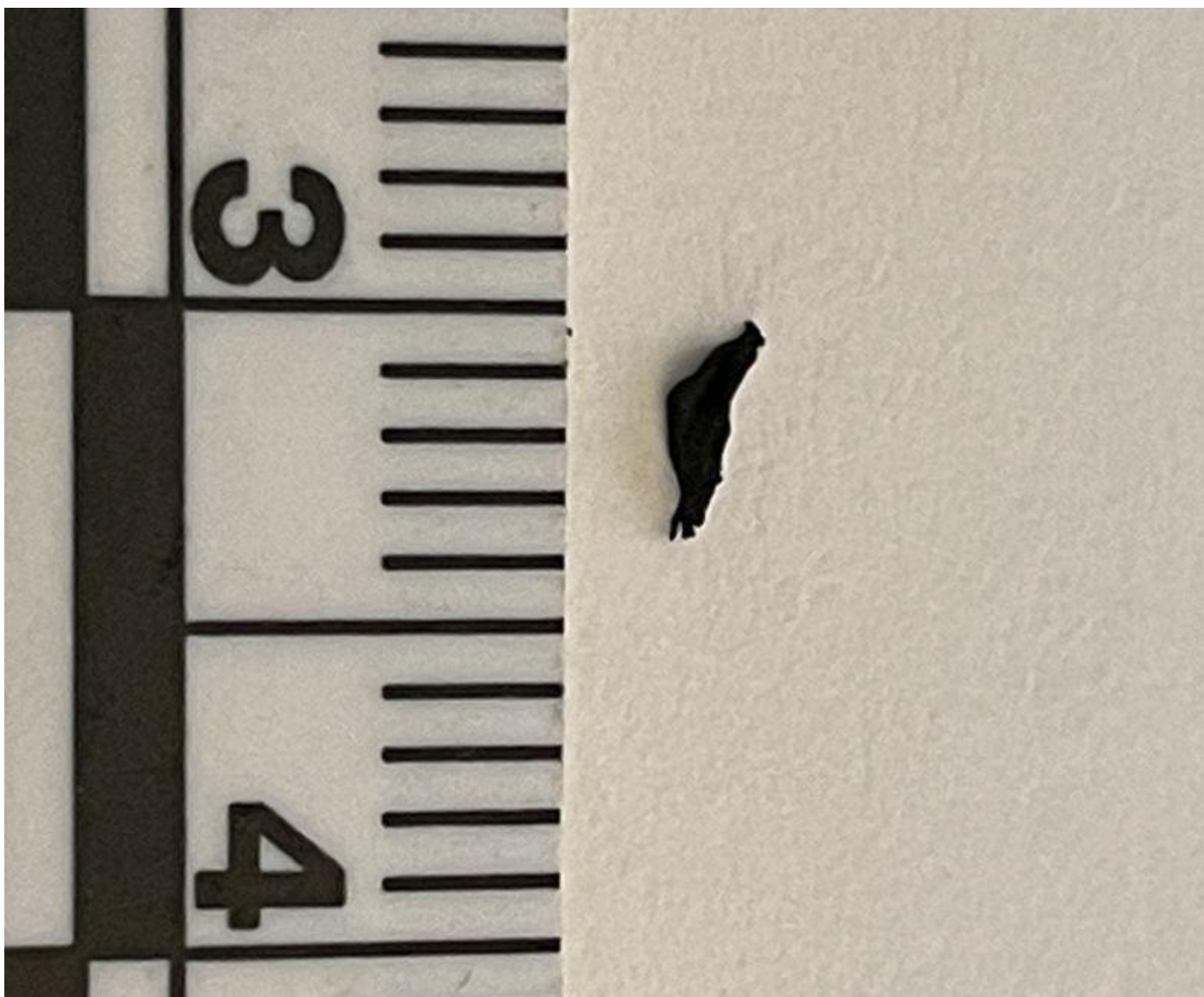
Photograph 6 - Fuel Pump Debris (NTSB Photo)
