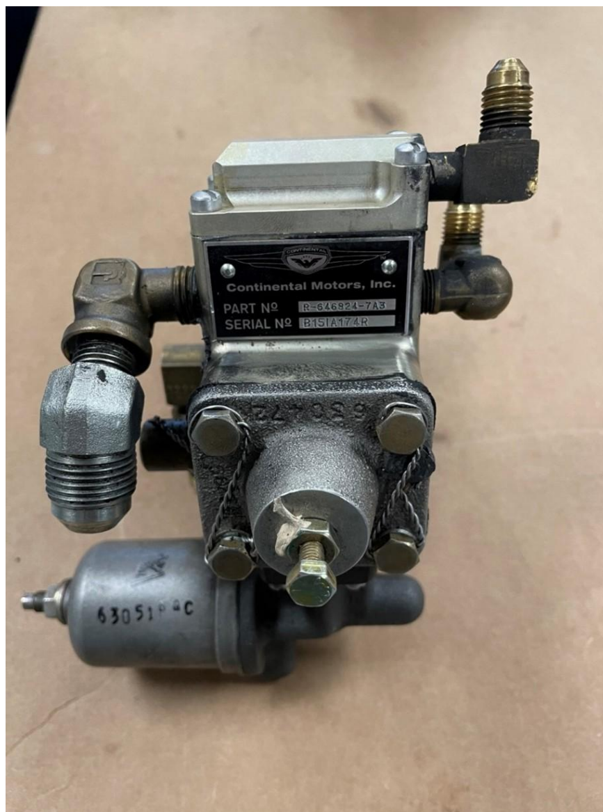
Photograph 5 Fuel Pump (NTSB Photo)
