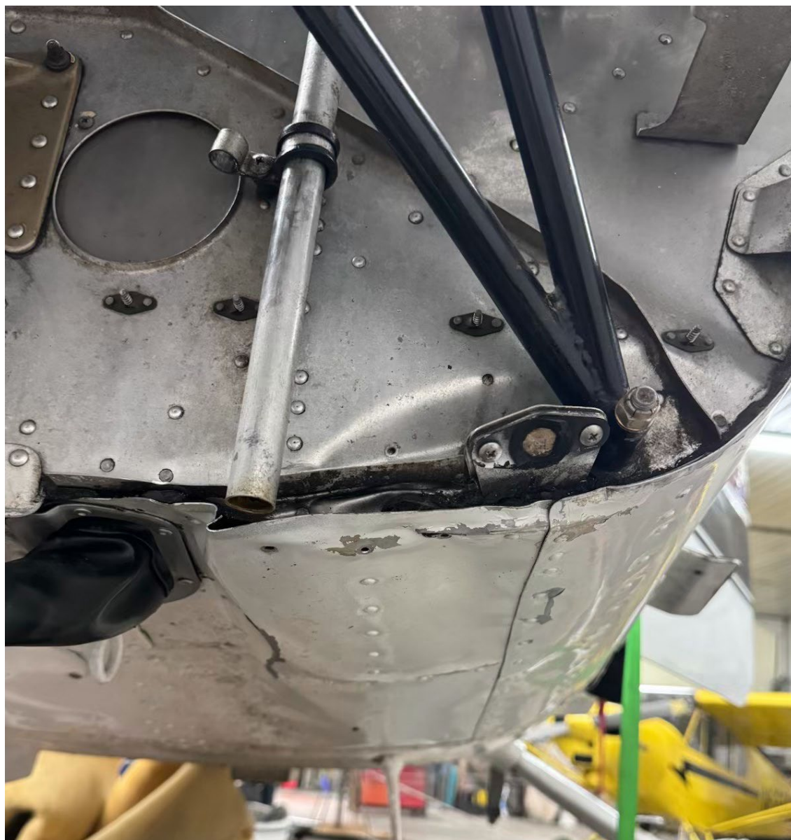
Photograph 3 - Damage to firewall and fuselage (Courtesy of FAA)
