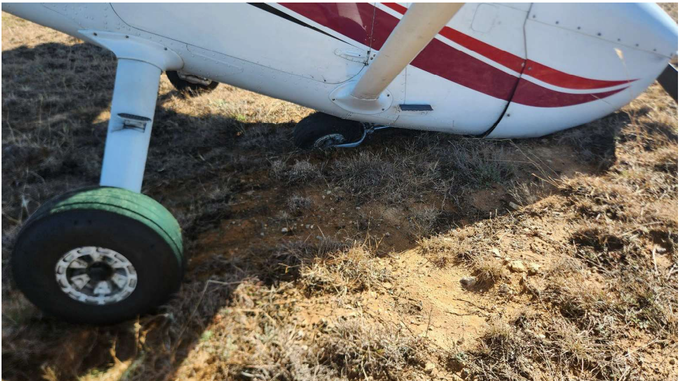
A closer look at the collapsed front landing gear.
