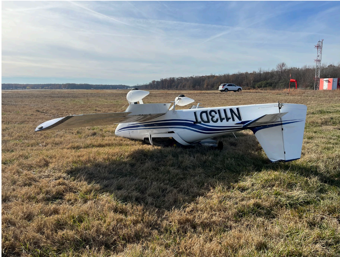
Photograph 2 - Substantial Damage to Vertical Stabilizer (Courtesy of FAA)
