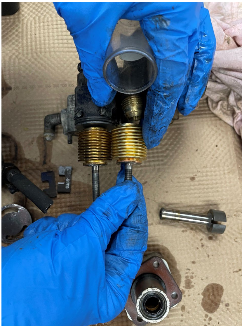
Photograph 4 - Fuel Pump Assembly Internal Aneroid (Courtesy of NTSB)
