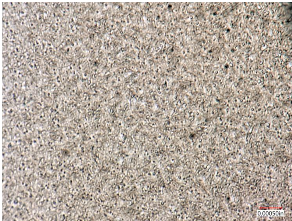
Figure 17. Typical EDS spectrum (top) and optical image from microstructure (bottom) of the fractured spring pin (P/N A-3150-18). 2 % Nital reagent as used for etching. The EDS pattern is typical for plain carbon and low-alloy steels. Microstructure appeared to be tempered martensite typical for plain carbon and low-alloy steels in the quenched + tempered condition. Mount Index No. 4637. Magnification: x720.
