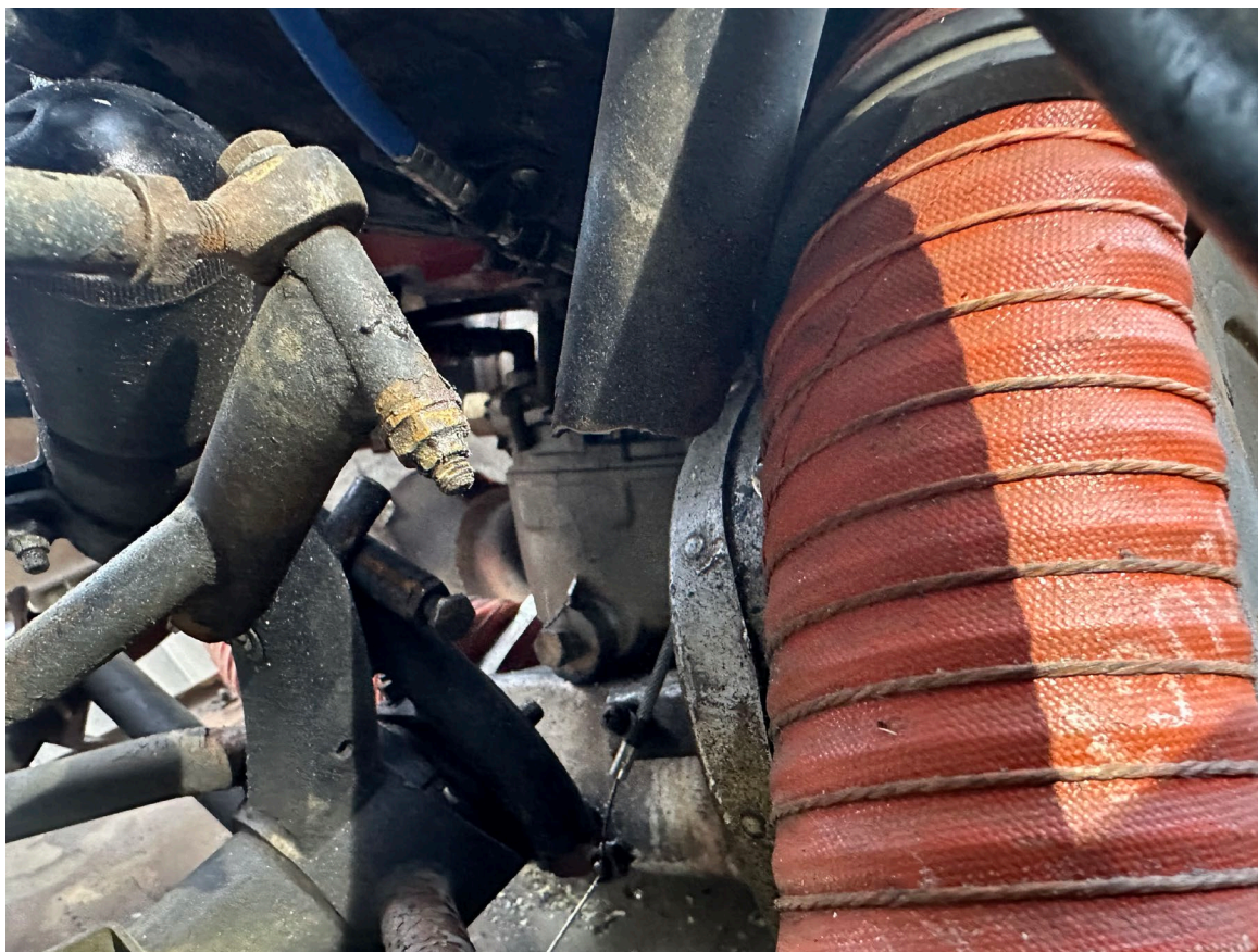
Photograph 4 - View of the fractured engine mount (Courtesy of Lubbock Aero)
