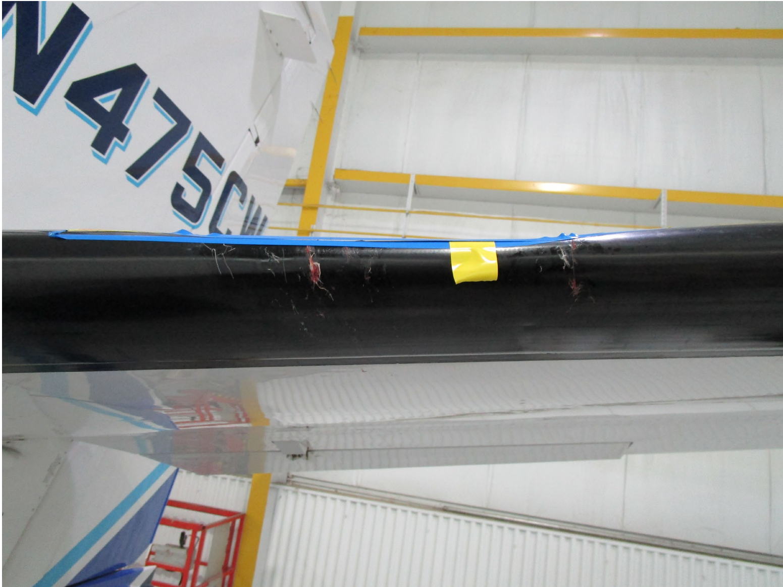
Photograph 1 - Left Horizontal Stabilizer Damage (Courtesy of Airplane Operator)
