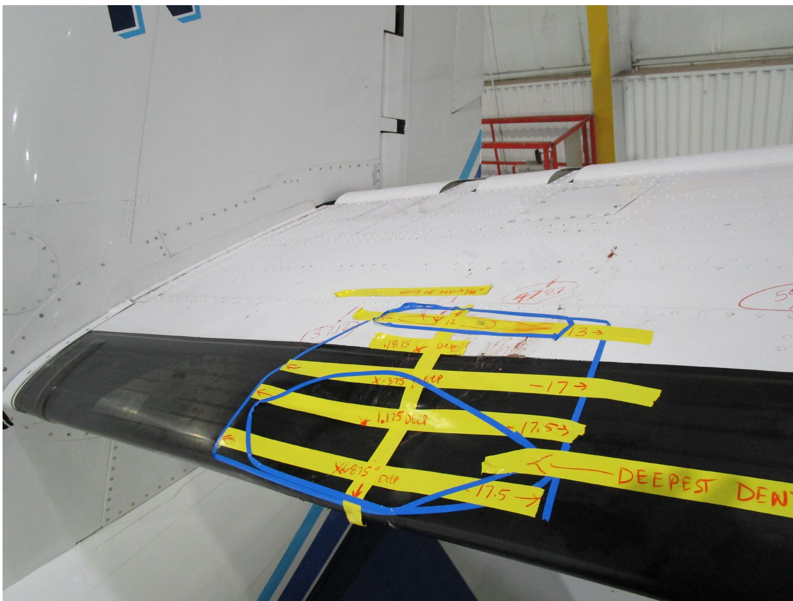
Photograph 2 - Upper Surface Damage of Left Horizontal Stabilizer (Courtesy of Operator)
