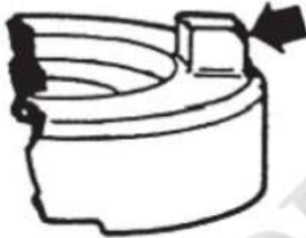
Figure 7-6. Worn Drive Lug
