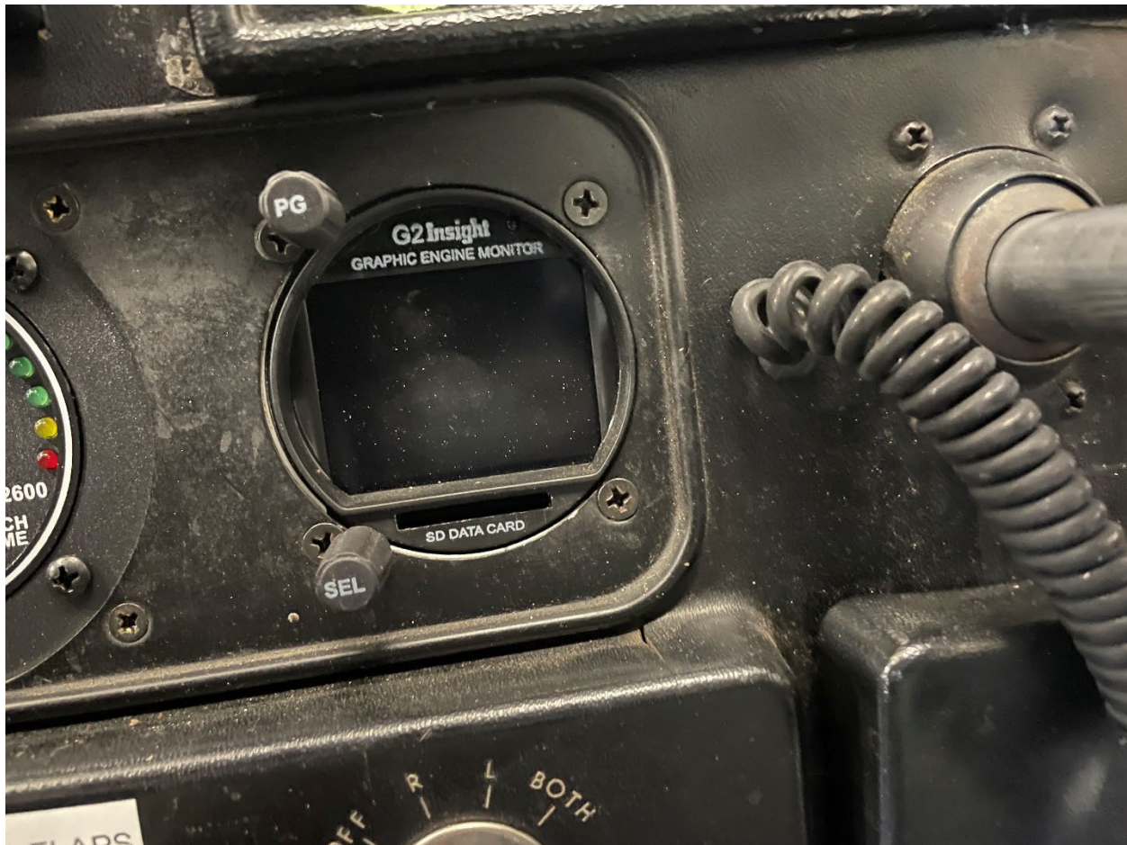
Insight G2 graphic engine monitor (SD card removed)
