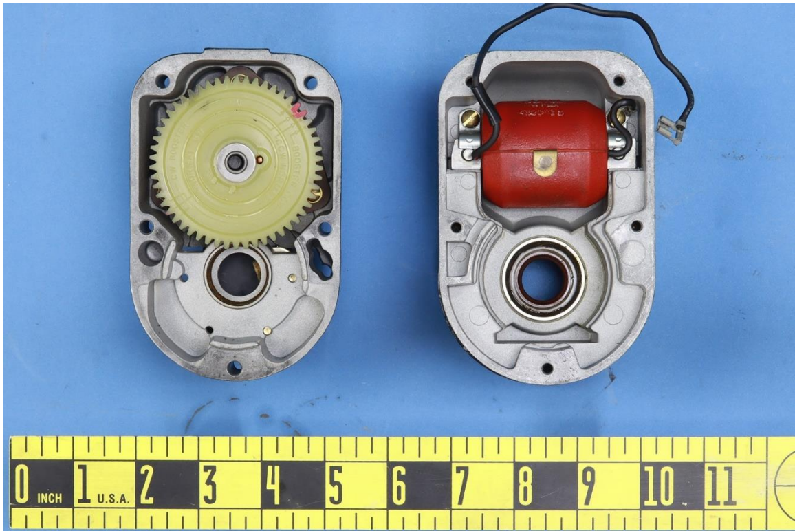
Figure 3. Left magneto after separating the housing.
