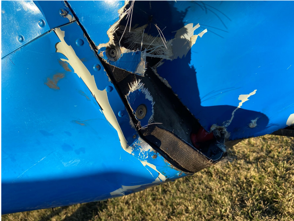
Photograph 2 - Lower Right Fuselage Damage (Courtesy of Pilot)
