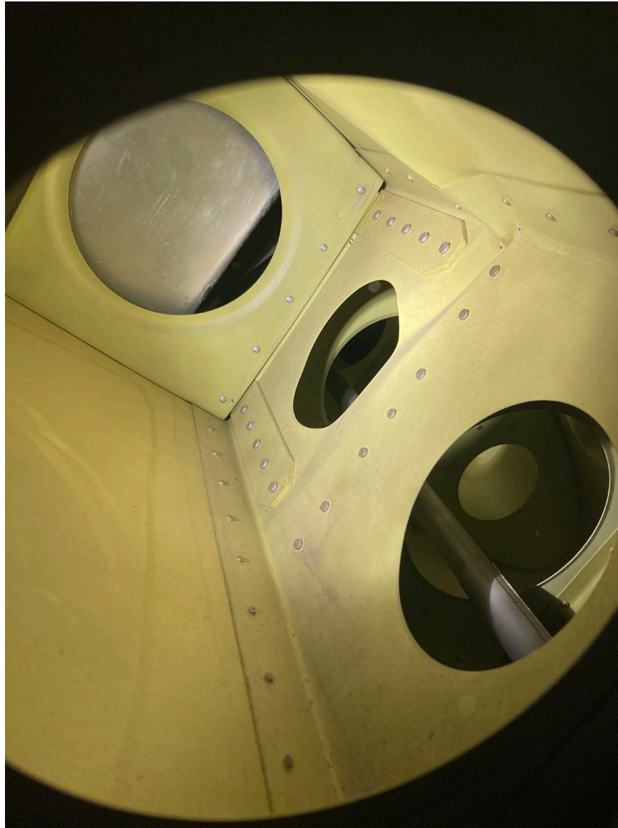
Photograph 4 - Deformation noted to right wing main spar (Courtesy of Airplane Owner)
