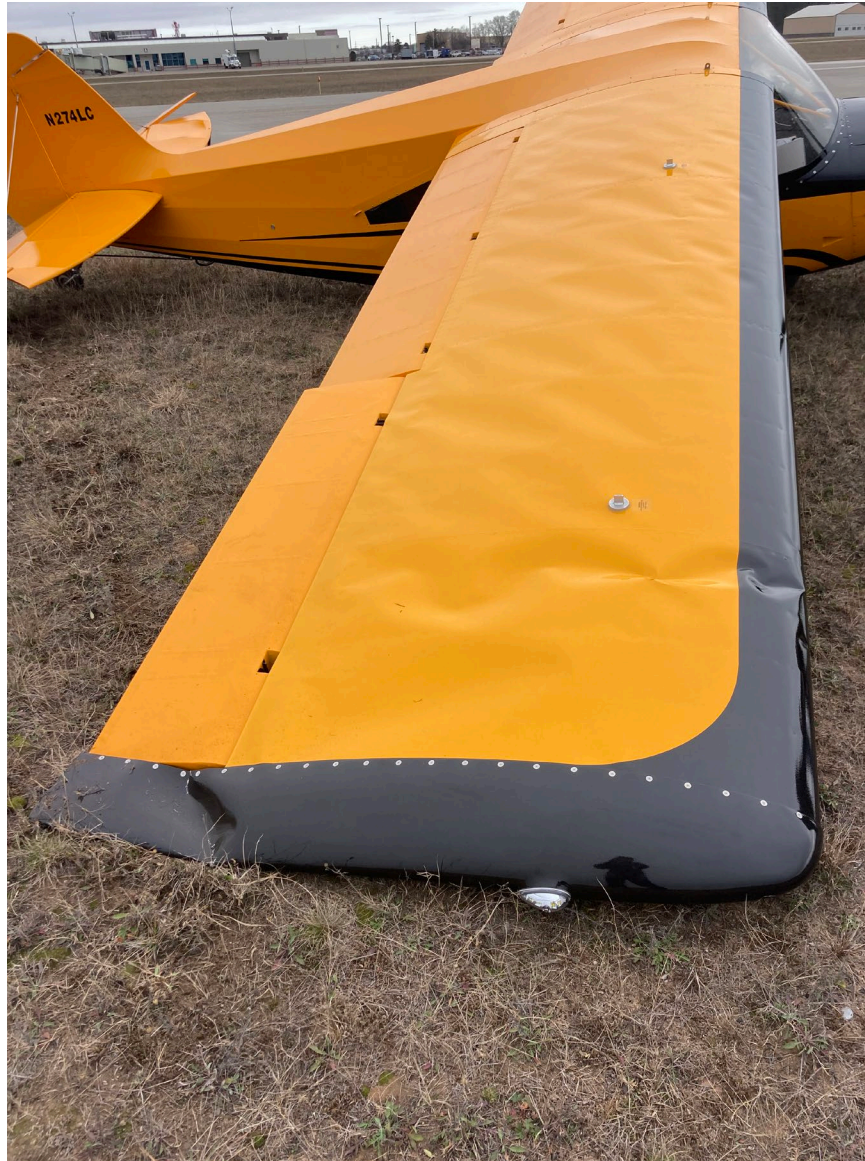
Photograph 3 - Deformation noted to right wing (Courtesy of Airport Manager)
