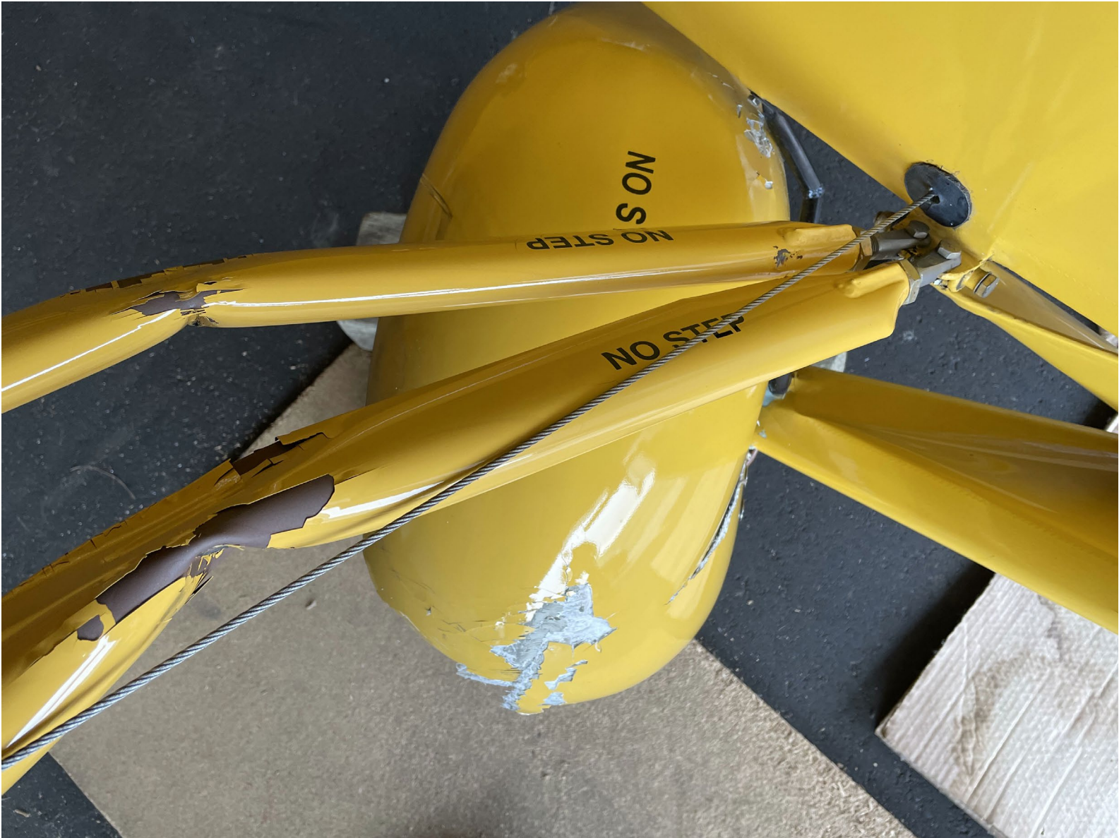
Photograph 3 - Top Down View Of Right Wing Lift Struts (Courtesy of FAA)
