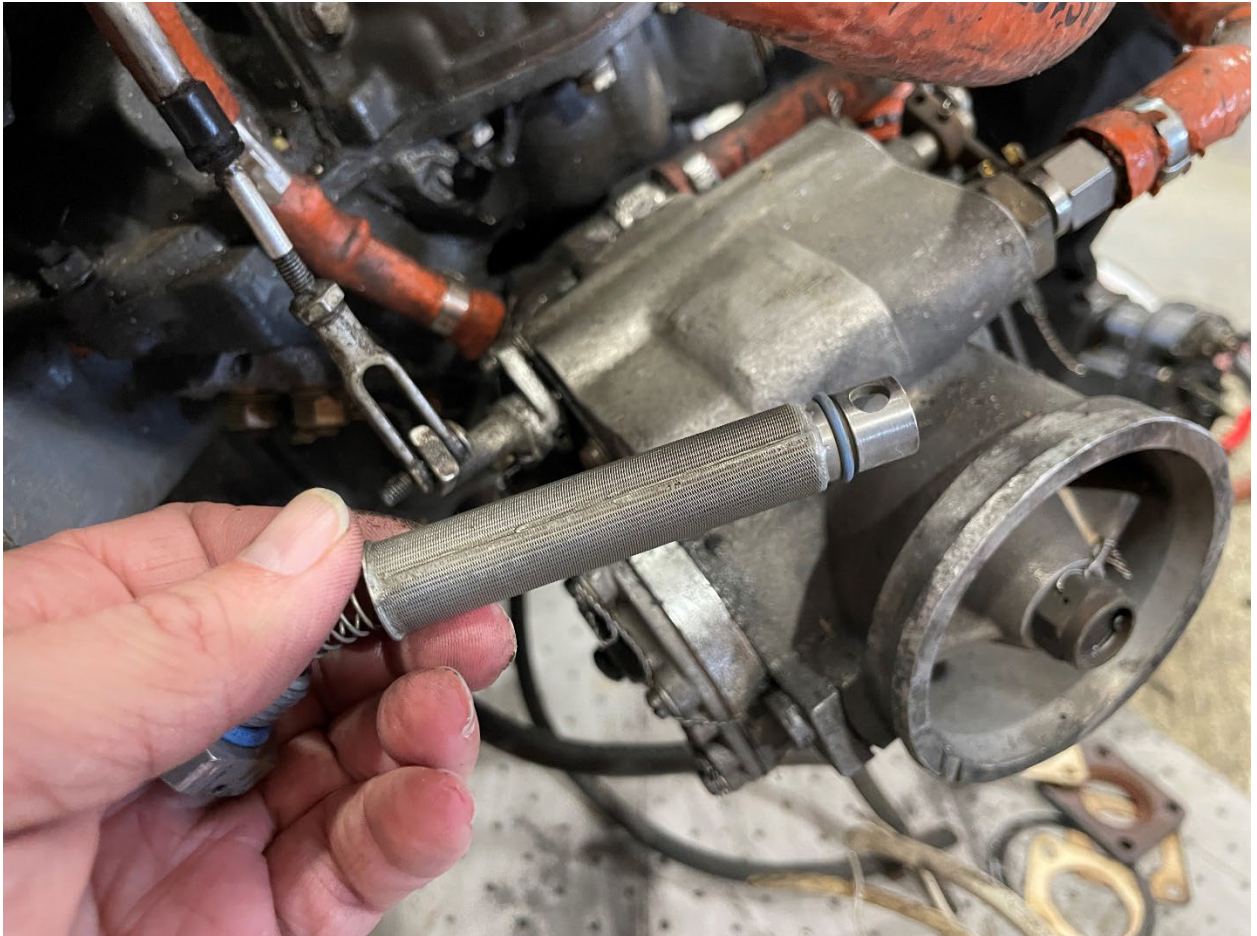
Figure 4 Inlet Fuel Screen (NTSB Photo)
