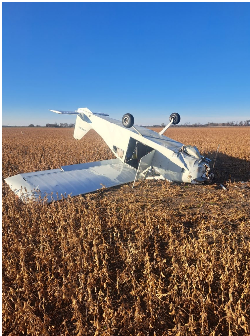
Photograph 2- Accident Airplane with Cowling Damage in Field (Courtesy of FAA)
