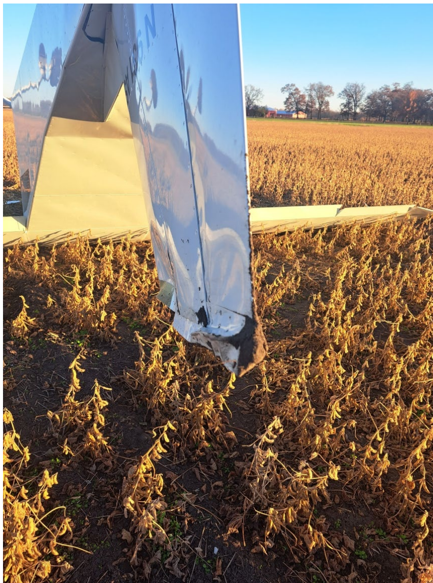
Photograph 2 - Accident Airplane with Damaged Vertical Stabilizer (Courtesy of FAA)
