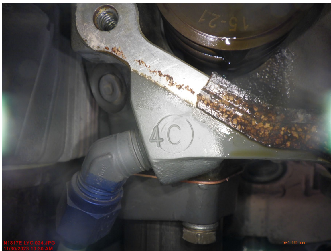
Photograph 5 - "C" Stamp on Number 4 Cylinder (Courtesy of Lycoming)
