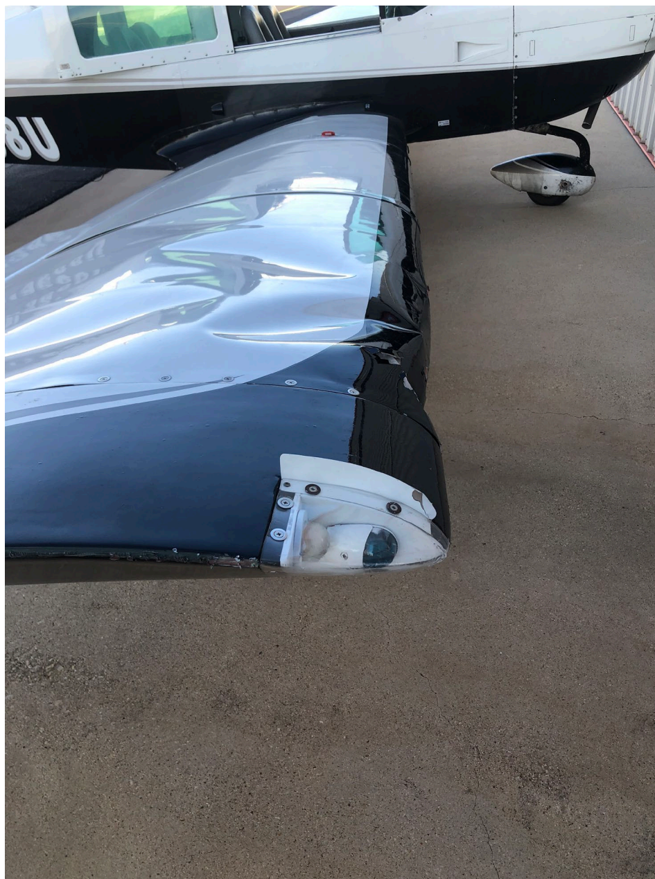
Photo 3 – View of the substantial damage sustained to the right wing (courtesy of the pilot).
