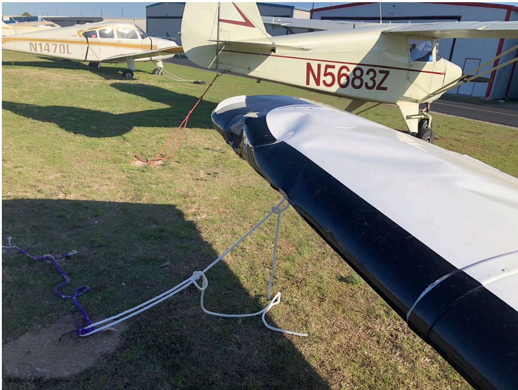
Photo 4 – View of the substantial damage sustained to the right wing (courtesy of the pilot).
