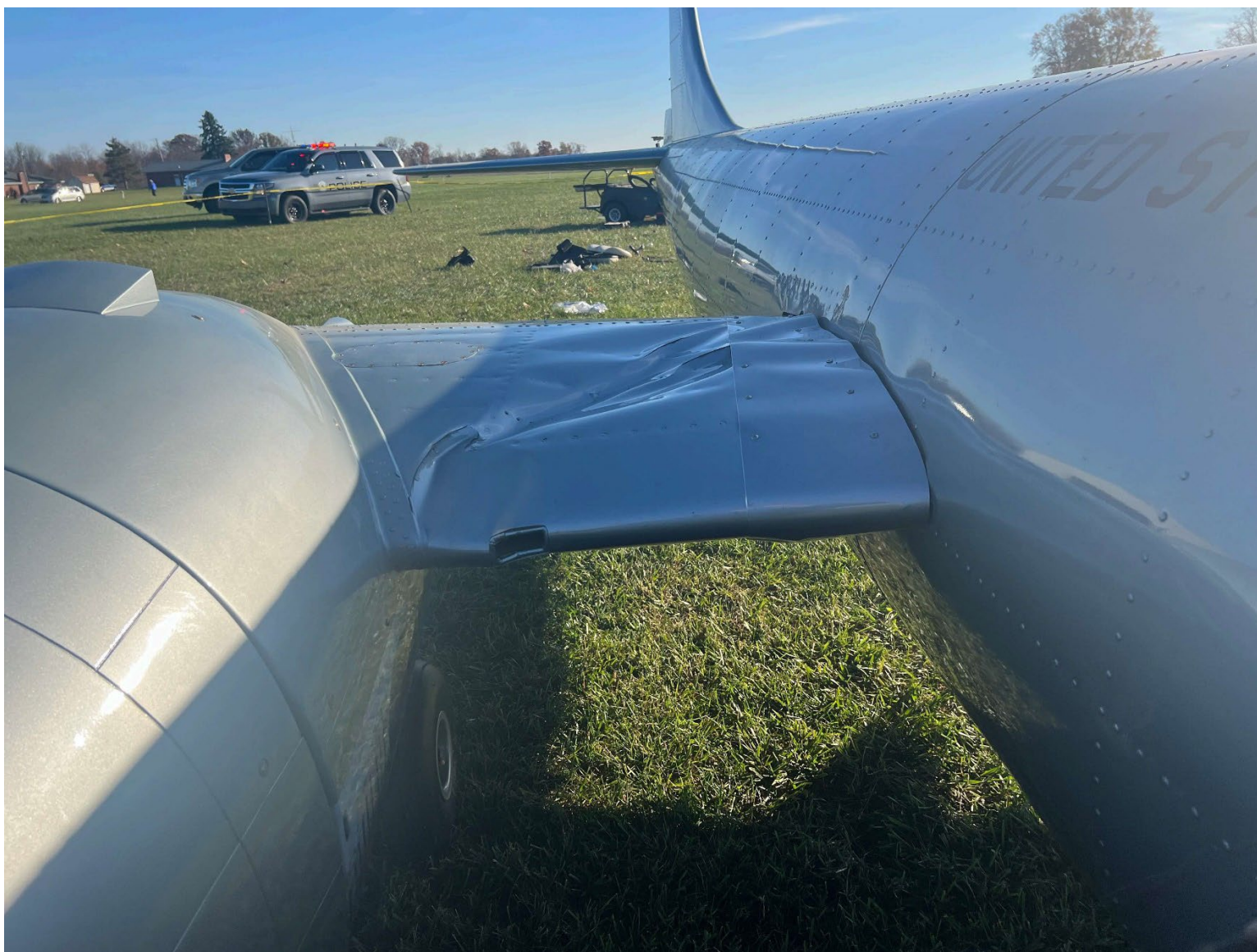
Photograph 3 - Right Wing Damage (Courtesy of Federal Aviation Administration)
