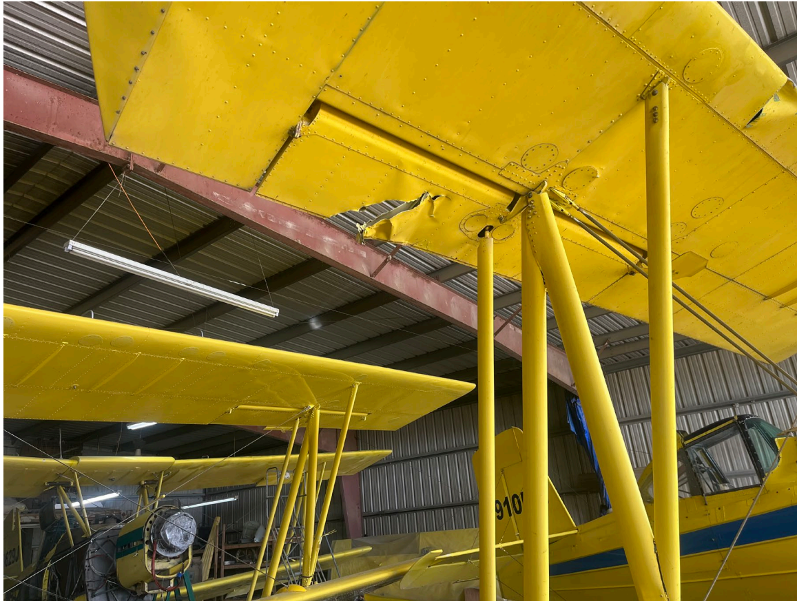
Photograph 3 - Upper right wing and aileron damage (Courtesy of FAA)
