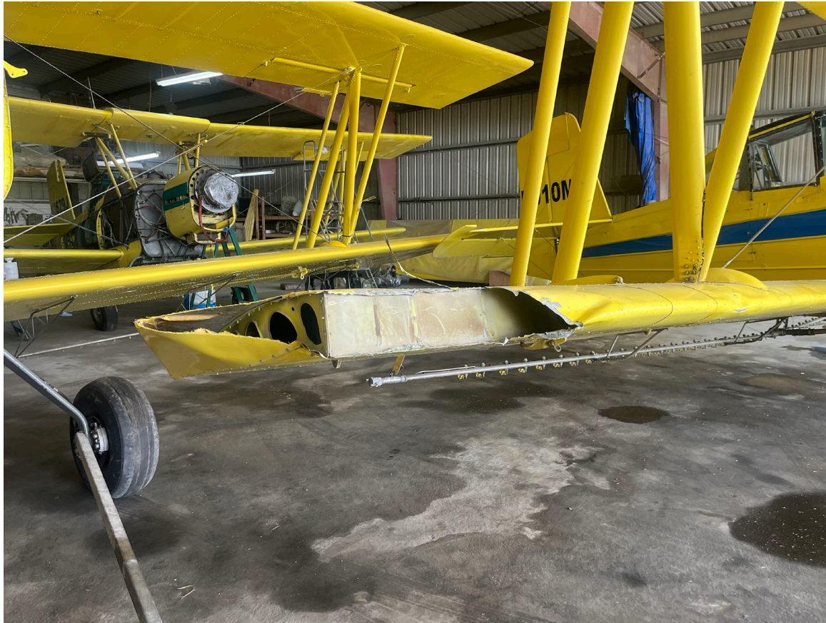
Photograph 2 - Lower right wing damage (Courtesy of FAA)
