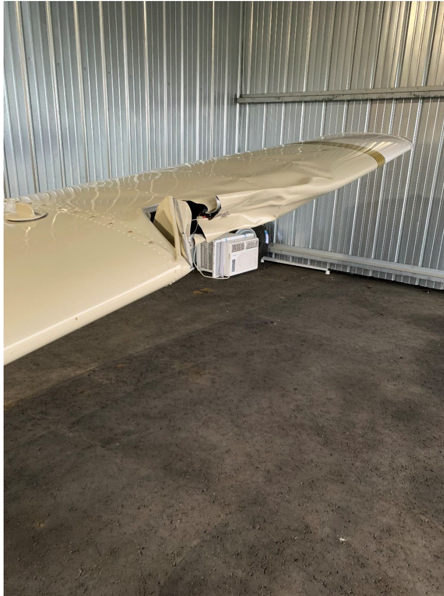
Photograph 1 - Damaged left wing (Courtesy of the Federal Aviation Administration)
