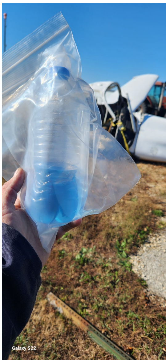
Photograph 5 - Fuel Drained from Left Fuel Tank (Courtesy of FAA)
