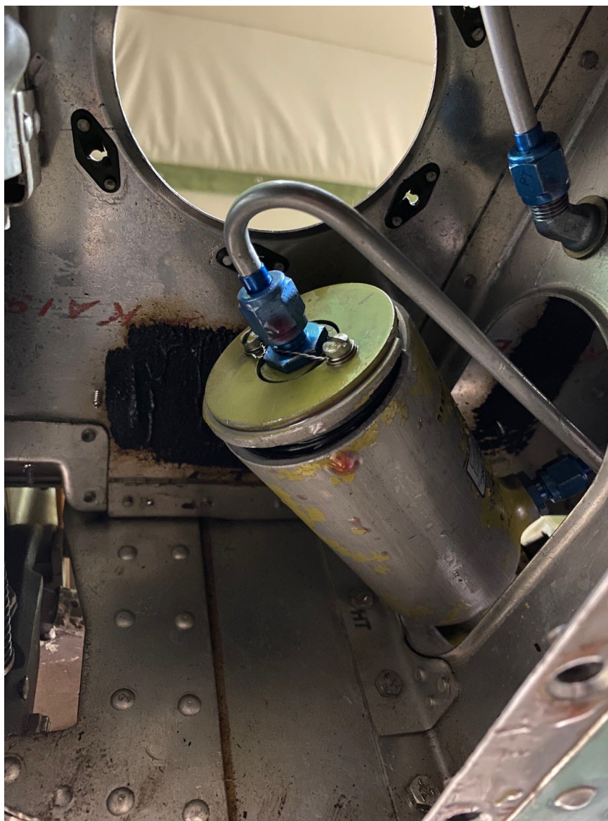
Photograph 2 - Fractured actuator (courtesy of pilot)
