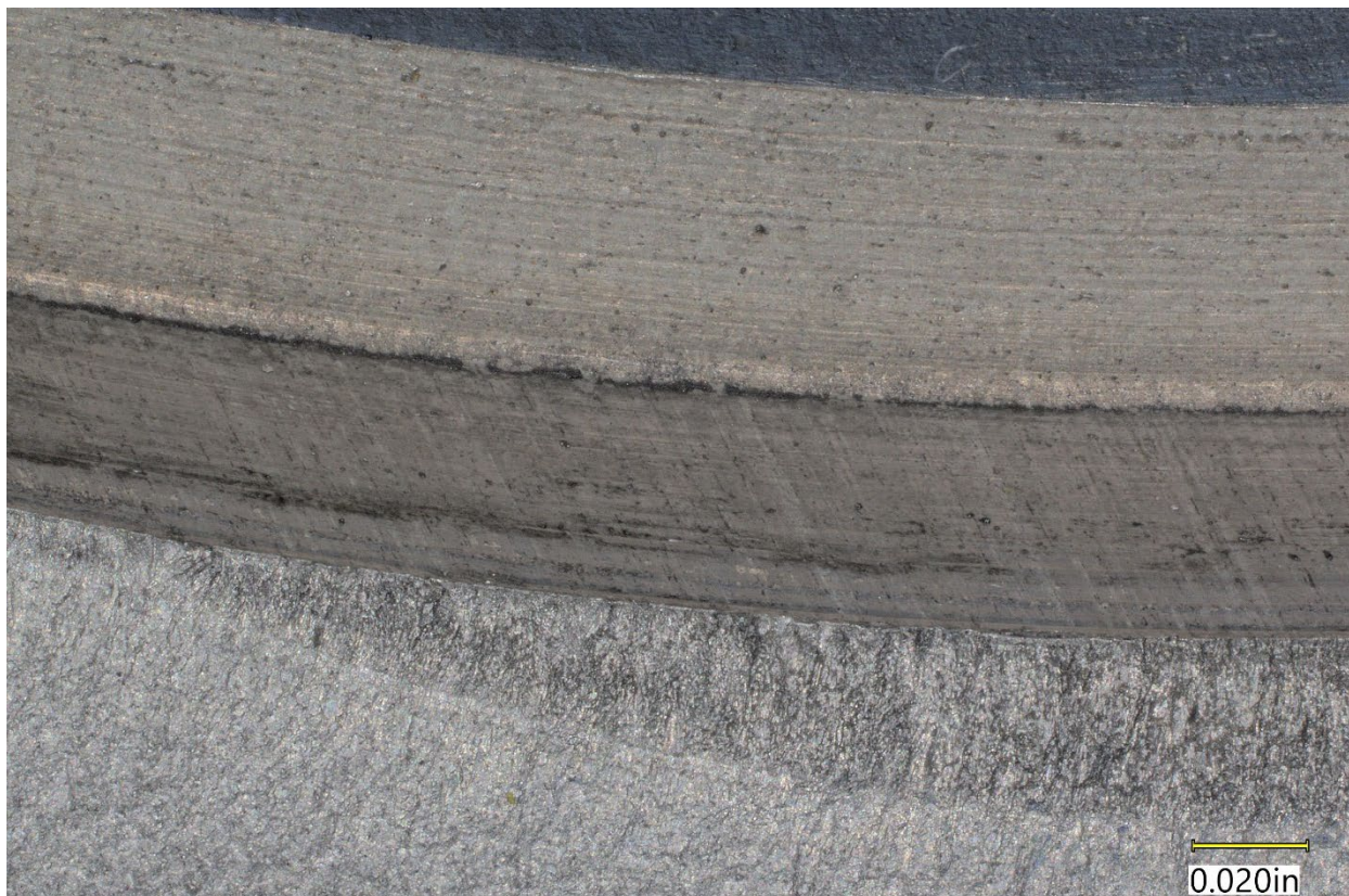
Figure 25. Additional cracking along the inboard corner of the groove opposite the fracture surface (lower portion).
