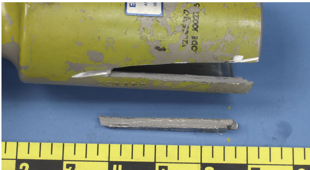
Figure 12. Mating faces of the longitudinal crack, after sectioning to open the crack faces.
