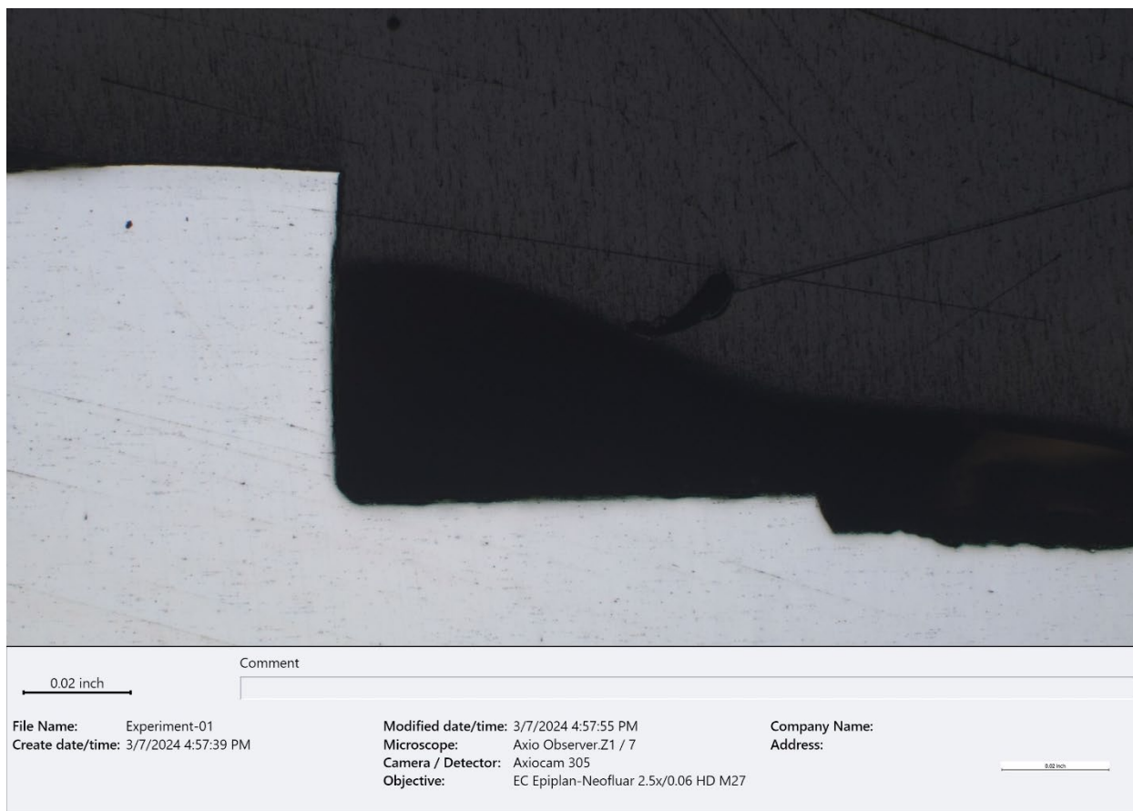
Figure 27. Bright-field (BF) optical metallograph cross-section of the actuator retaining ring showing an angled crack propagating from the left groove radius (~25X, as polished).
