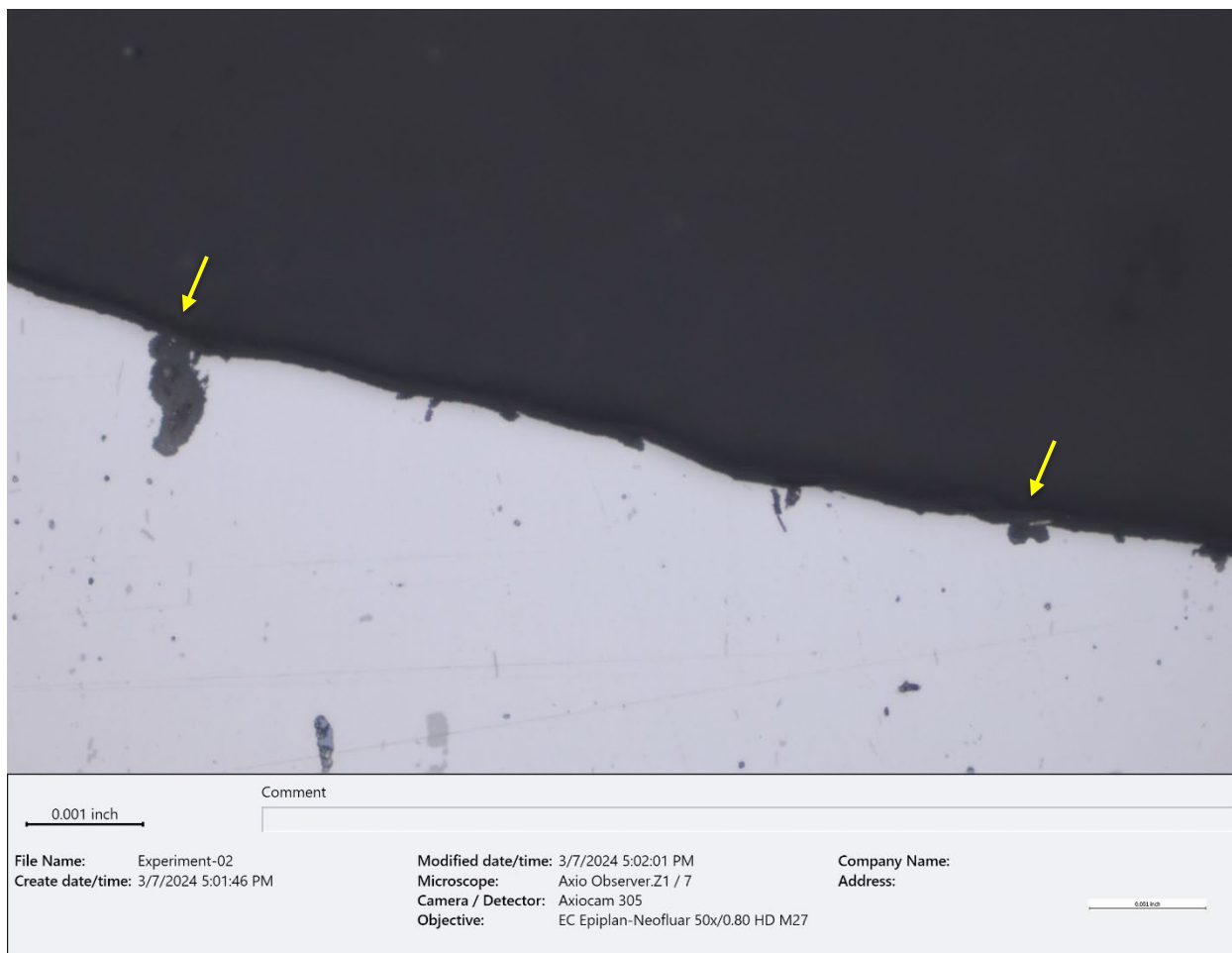
Figure 28. BF optical metallograph showing a closer view of corrosion pits from the lower groove surface in Figure 27 (~200X, as polished).
