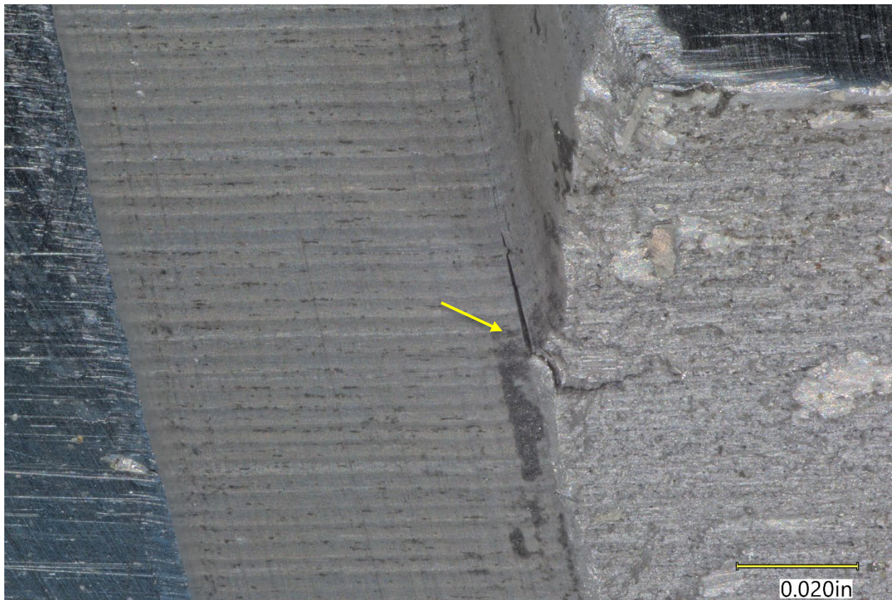
Figure 24. View of the secondary crack off the outboard groove corner, opposite angle showed in Figure 25. The crack is identified by the yellow arrow.
