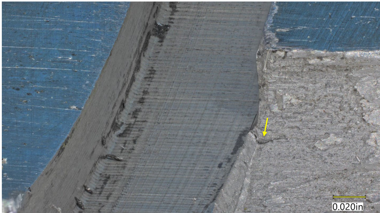
Figure 23. View of the clip groove, showing cracking (arrow) along the corner with the separated mating fracture surface.
