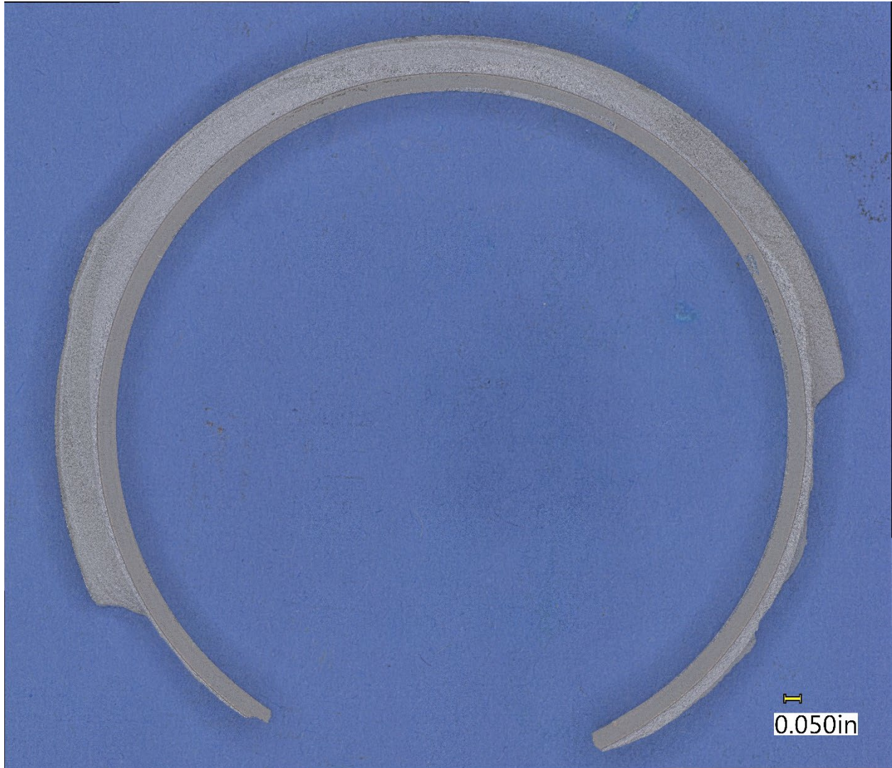
Figure 10. Montage of magnified images of the crack face of the circumferential crack, showing indications of progressive cracking.
