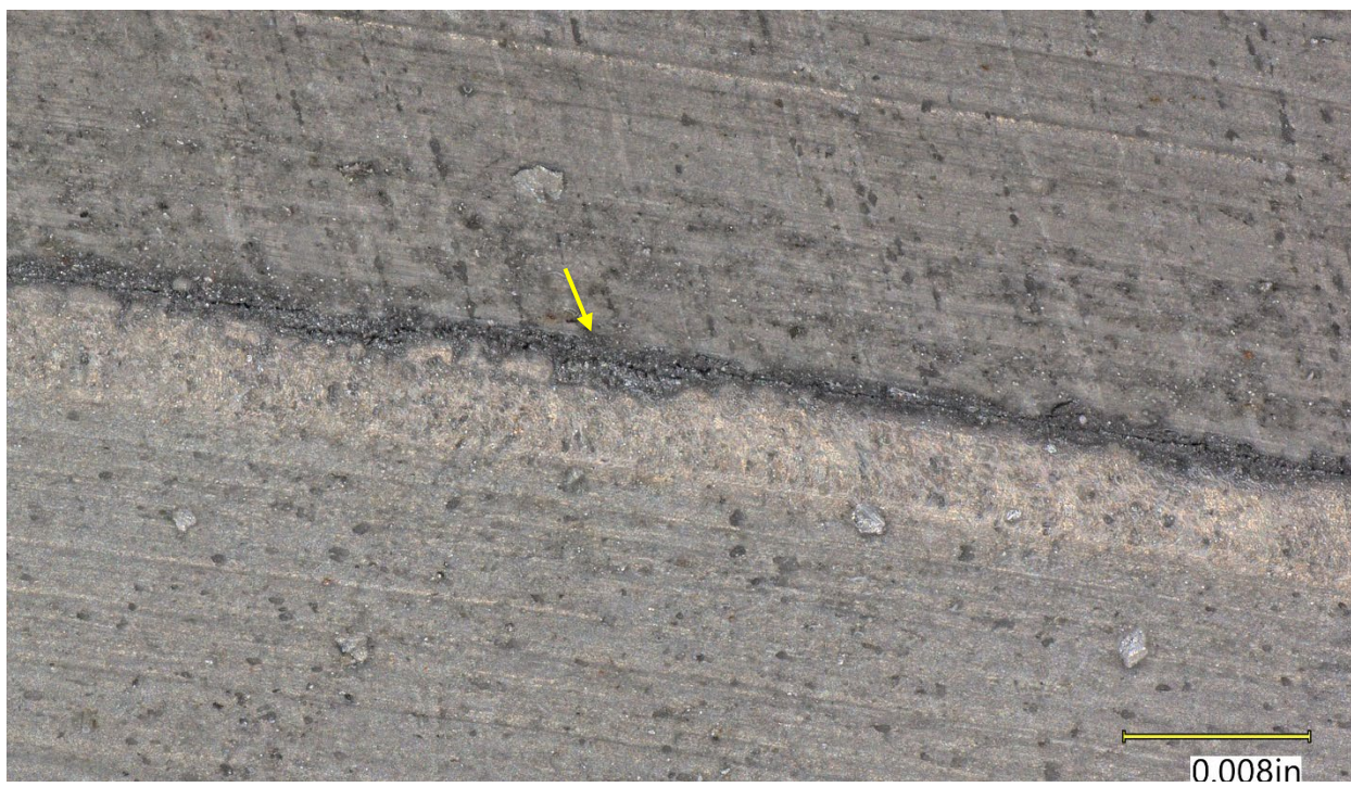
Figure 26. Closer view of the inboard corner cracks, collocated with pitting (dark).
