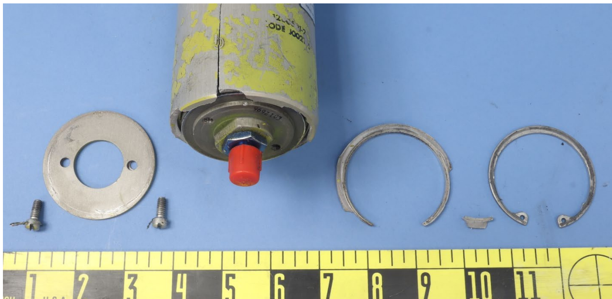
Figure 7. The cracked end of the actuator pictured in Figure 4, after removal of the screws and the end cap.
