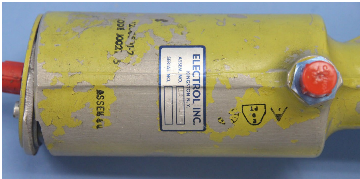
Figure 3. View of the markings on the housing barrel of the actuator, with the circumferential crack on the right.
