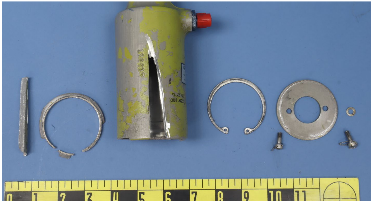
Figure 8. The cracked end of the actuator pictured in Figure 7a, after sectioning and removal of the cracked regions of the housing barrel.
