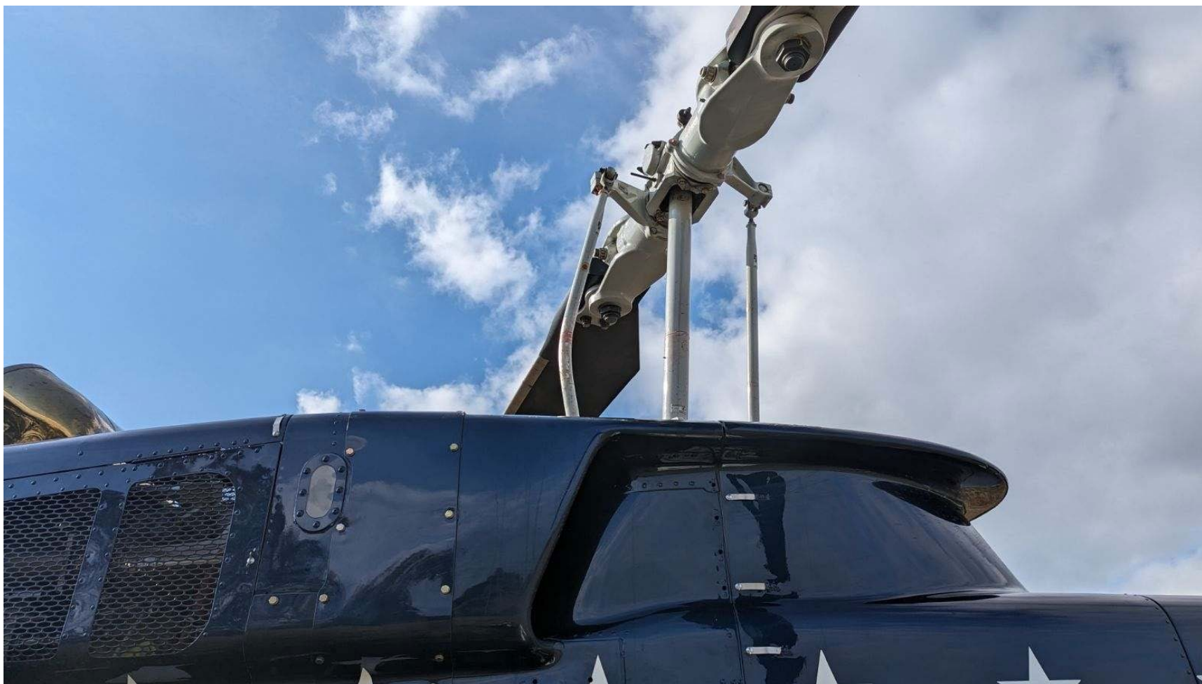
Photograph 1 - Pitch Change Link Damage (Courtesy of the Operator)
