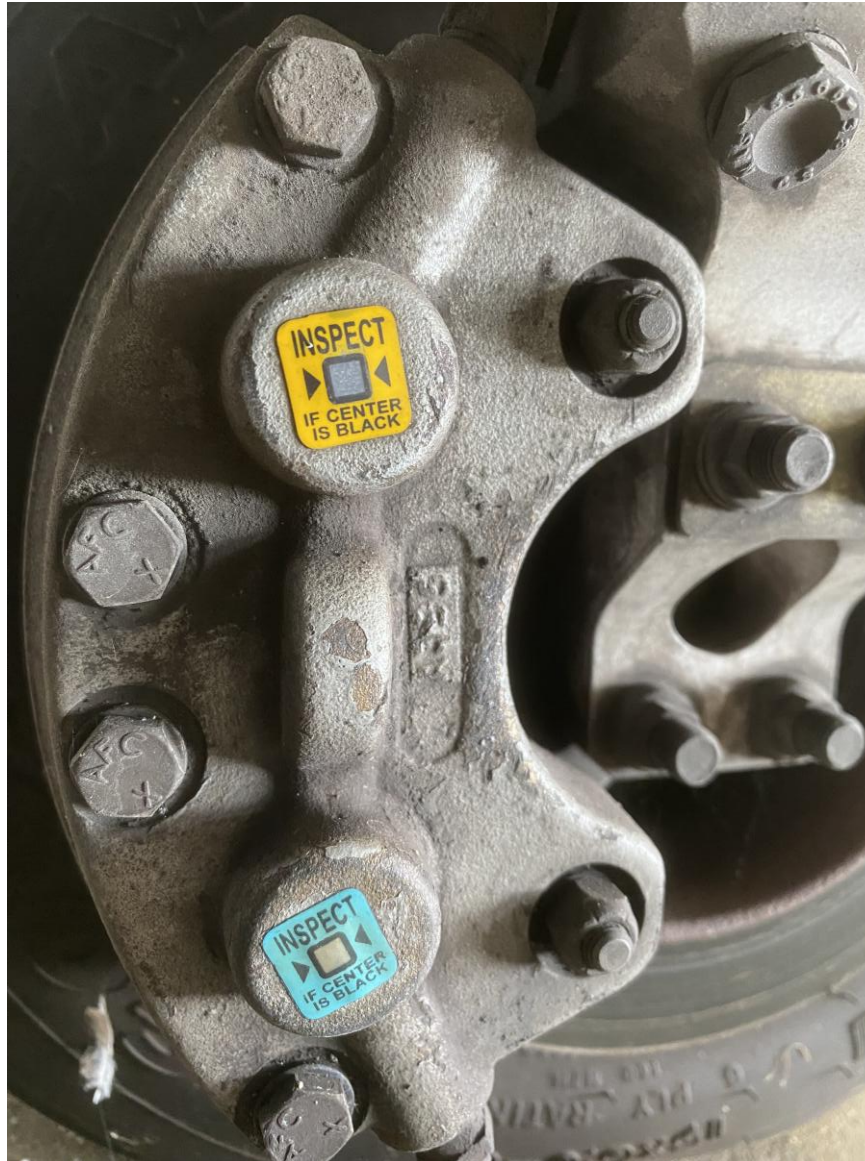
Photograph 6 - Left Brake Assembly with Temperature Indicators (Courtesy of Airplane Owner)
