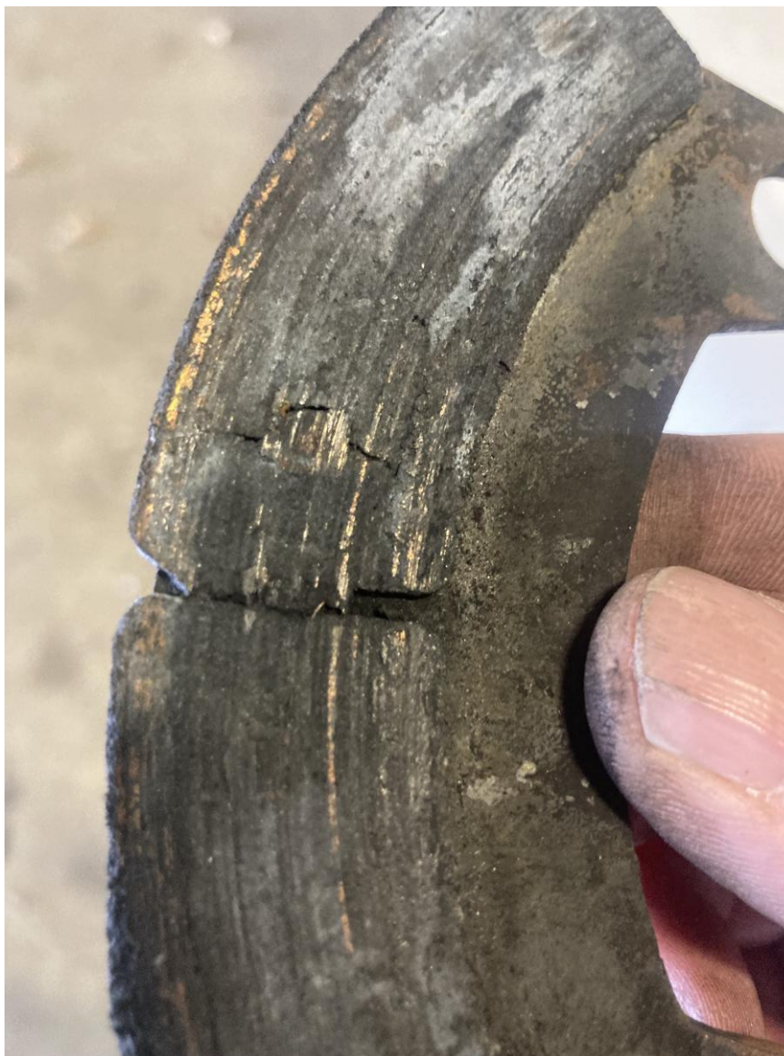
Photograph 5 - Right Brake Linings (Courtesy of Aviation Mechanic)
