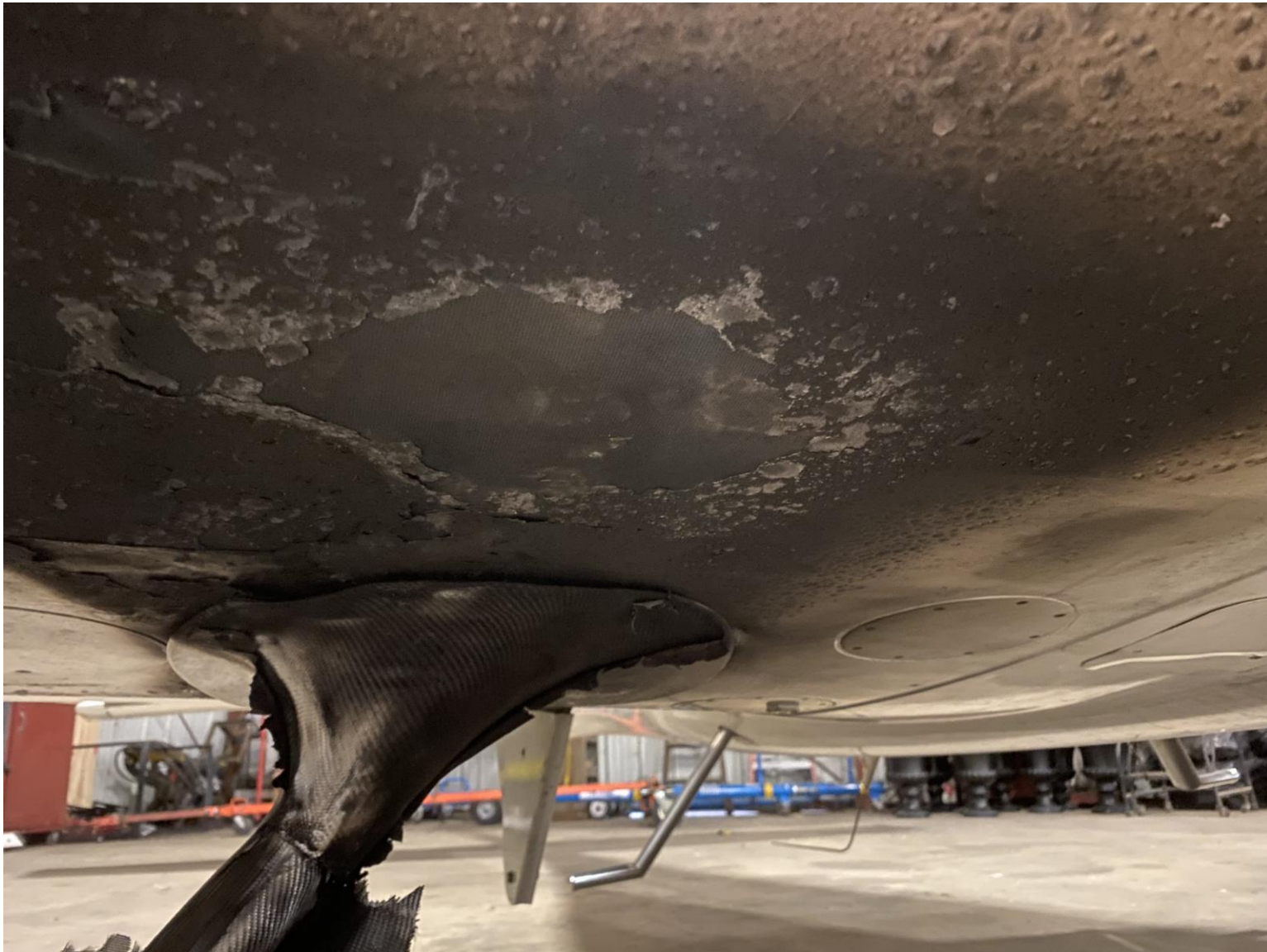
Photograph 3 - Fire Damage to Lower Right Wing (Courtesy of Airplane Owner)
