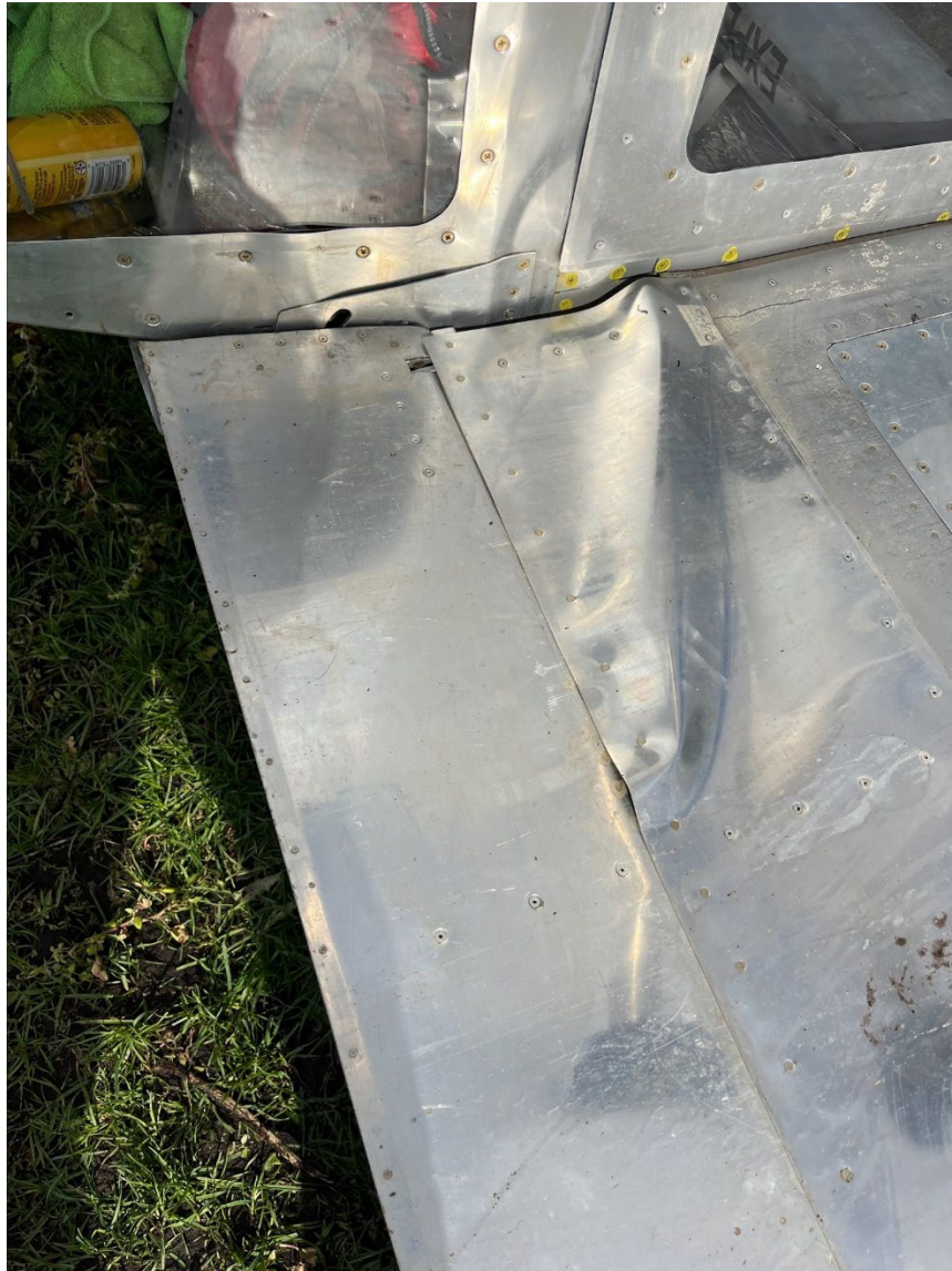
Photograph 3 - Left Wing Damage (Courtesy of the Federal Aviation Administration)
