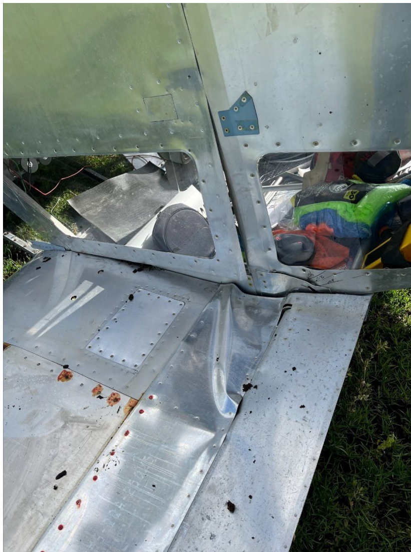
Photograph 2 - Right Wing Damage (Courtesy of the Federal Aviation Administration)
