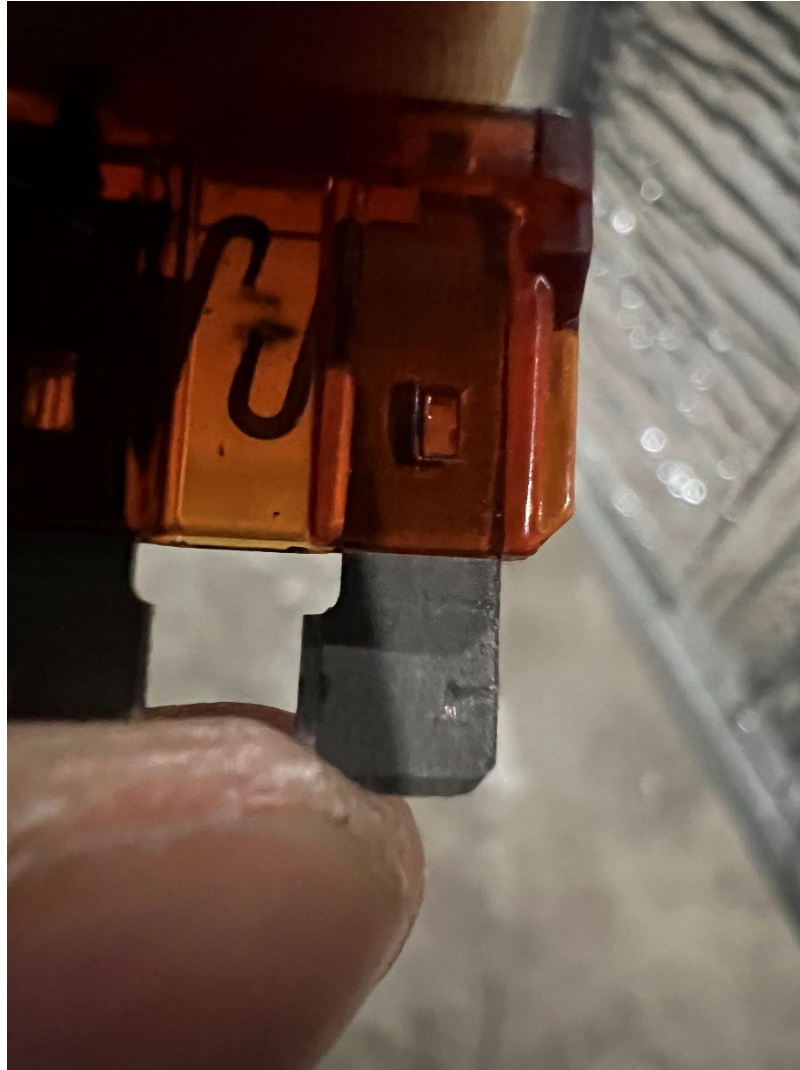
Photograph 4: Blown Fuse (Courtesy of the Pilot/Aircraft Owner)
