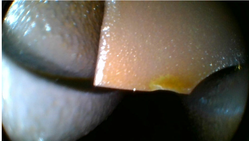
Figure 5. Broken Turbocharger Turbine Blade
