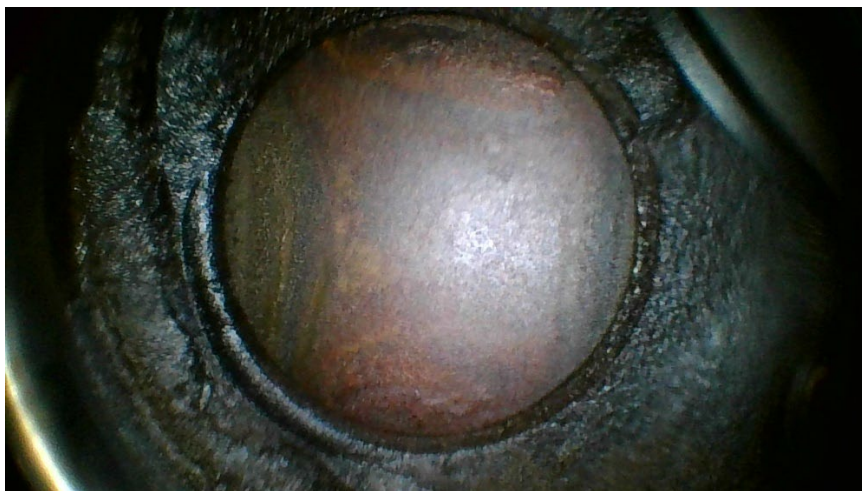
Figure 4. #6 Cylinder Exhaust Valve Face
