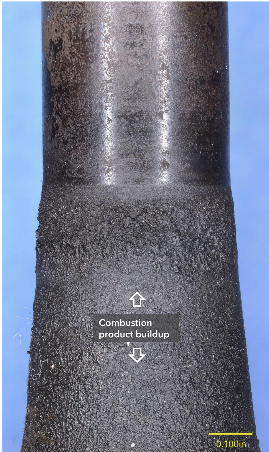
Figure 4. Buildup of combustion products on the number 4 exhaust valve stem outside the area that engaged the valve guide.
