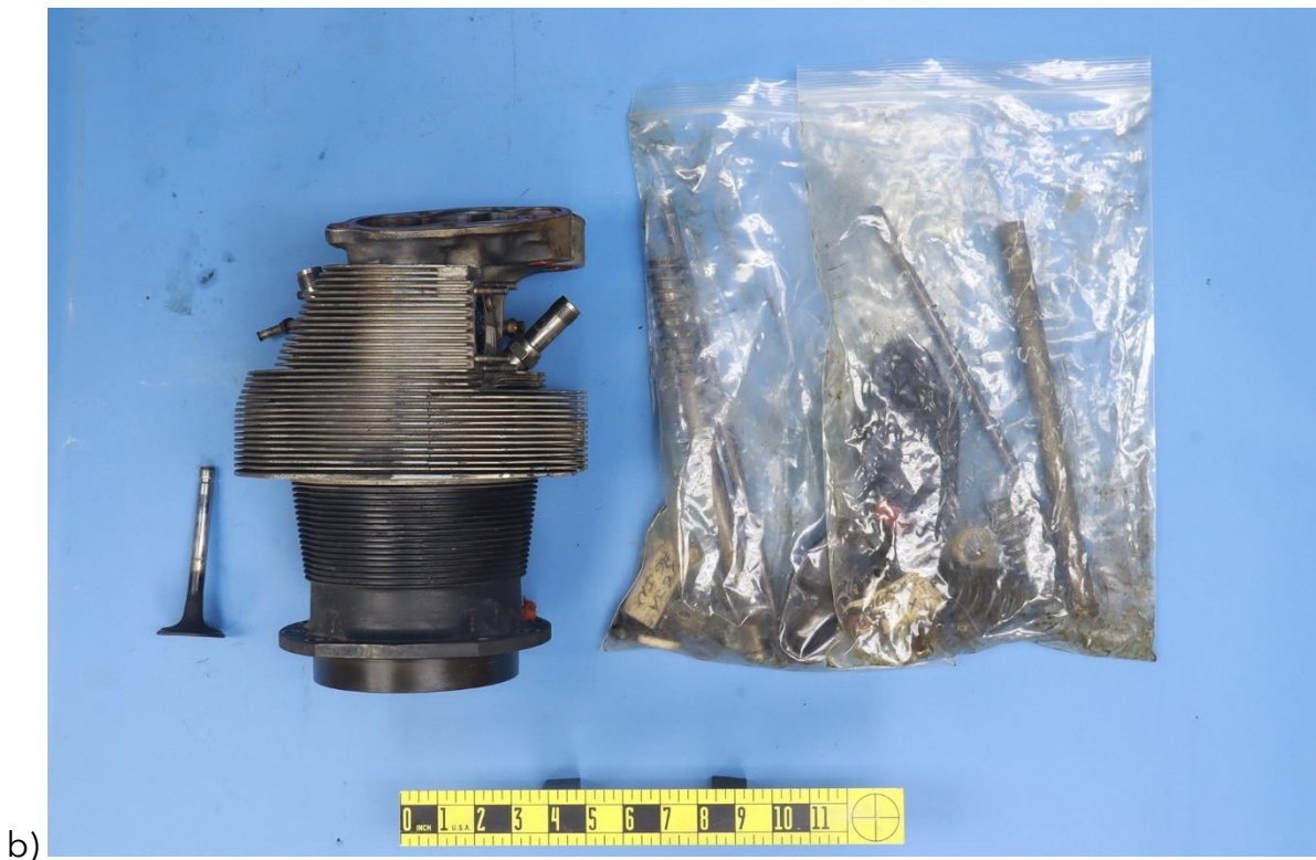
Figure 1. Exhaust valves and cylinder assemblies with intake and exhaust valve train components: a) number 4 and b) number 6.
