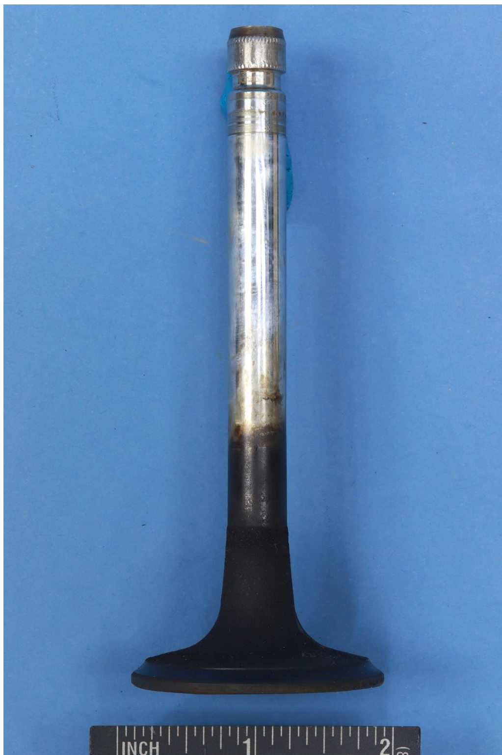
Figure 7. Images of number 6 exhaust valve: a) overall image;
