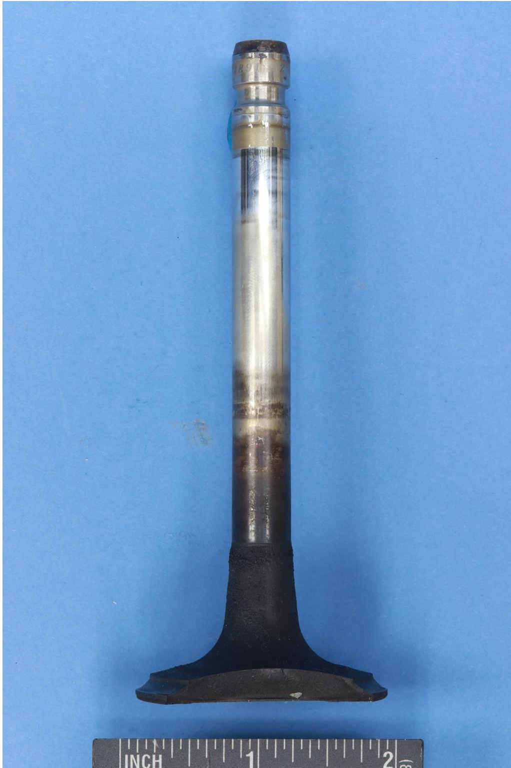
Figure 2. Number 4 exhaust valve: a) stem and fractured valve head and
