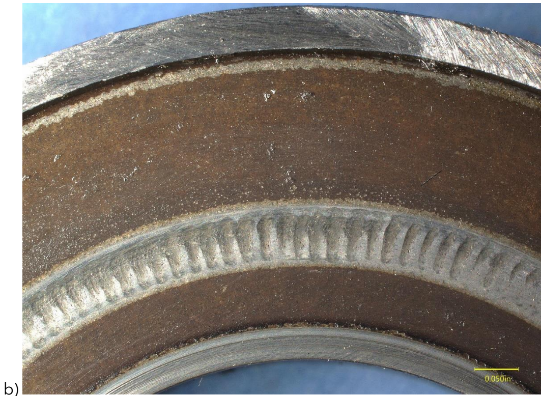
Figure 10. Number 6 exhaust valve rotocoil: a) post-disassembly and b) wear of flat race leaving behind impressions of the spring.
