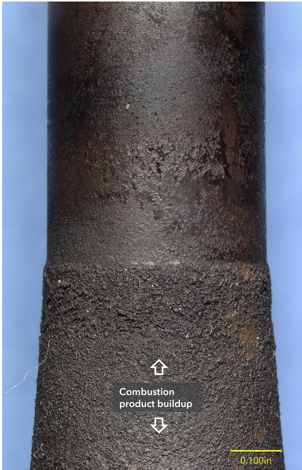
Figure 8. Number 6 valve stem showing buildup of combustion products outside the area that engaged the valve guide.
