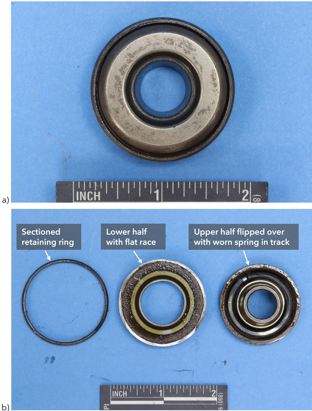
Figure 6. Number 4 exhaust valve rotocoil: a) As received before disassembly; b) post disassembly;
