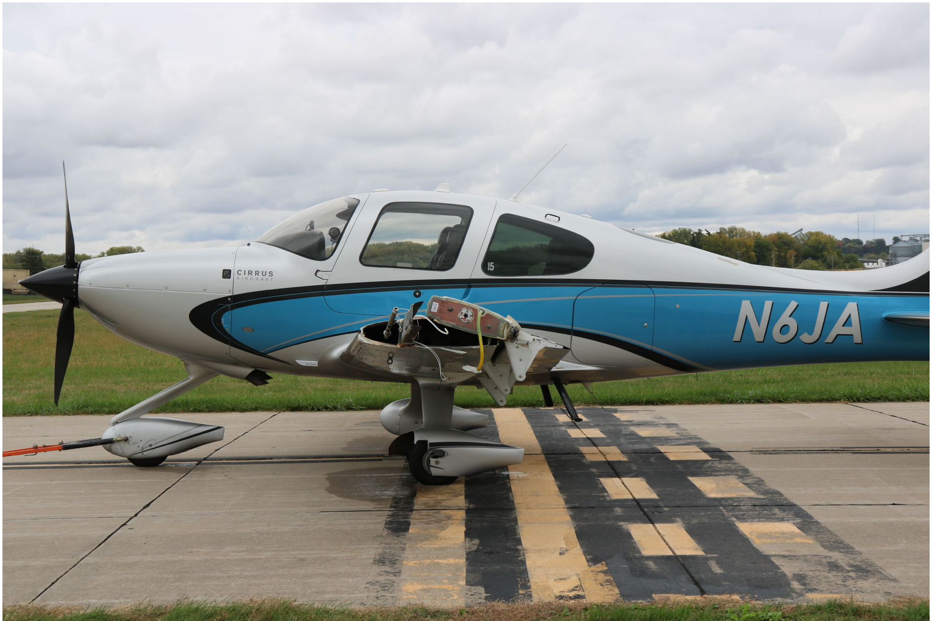
Photo 1 – View of Aircraft with Left Wing Damaged, Photo Courtesy of Airport Operations
